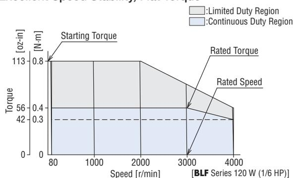
The specified speed is compared against the feedback signal to adjust the motor supply voltage and frequency, in order to stabilize the speed.
