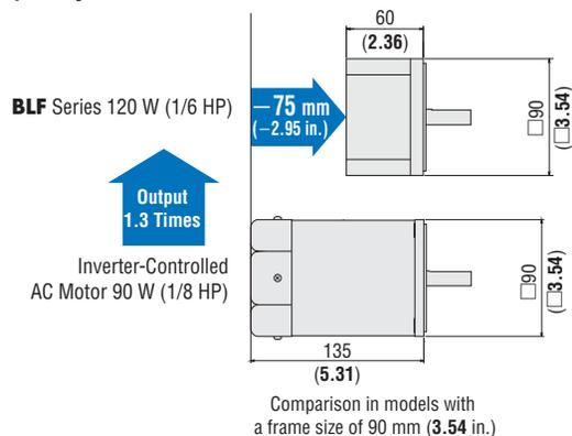
The compact yet powerful motor incorporates permanent magnets in the motor rotor. Compared with an AC motor having a frame size of 90 mm (3.54 in.), a brushless motor of the same specifications is 75 mm (2.95 in.) shorter and offers 1.3 times more output.
