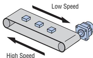
Because of the different motor structure and control method, speed control range of the brushless motor is wider than that of the AC speed control motor.
