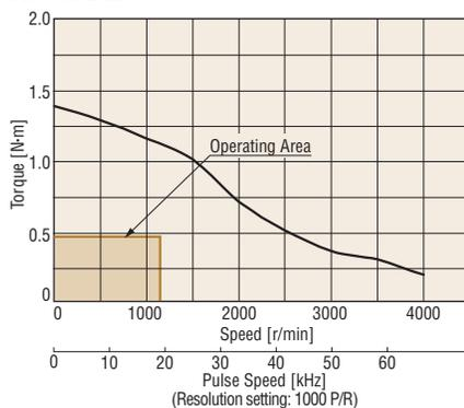
Select a motor for which the operating area indicated by operating speed and required torque falls within the pullout torque of the speed – torque characteristics.
