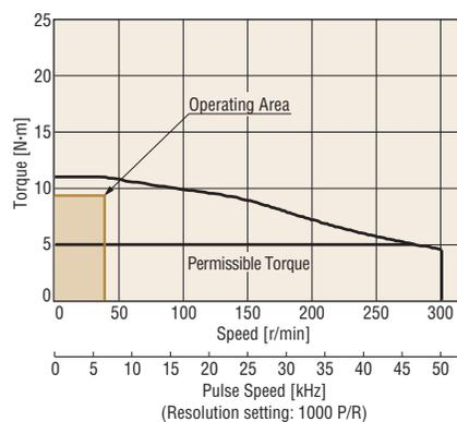
**PN** geared type can operate inertia load up at starting/stopping to acceleration torque less than maximum torque.
