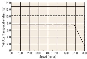
\* For X-axis, the maximum speed read from the graph is limited by the stroke. Check the maximum speed for each stroke in **EZSII** Series products.
