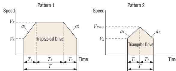
$V_{Rmax}$  : Calculated maximum speed of triangular drive [mm/s]
