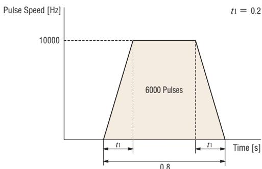
④ Calculate the operating speed  $N_M$  [r/min]
