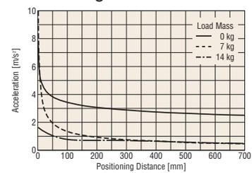
● **EZS4D□-A/EZS4D□-C** (Lead 12 mm, Single-Phase 100-115 VAC/Single-Phase 200-230 VAC)
