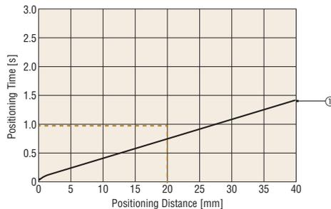
The above graph shows that the load can be positioned over 20 mm within 1.0 second.
