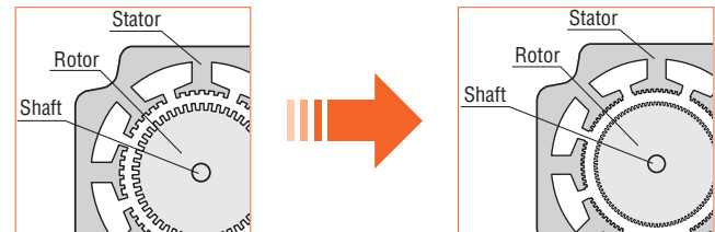
Step Angle 1.8° Standard Type (50 teeth)
