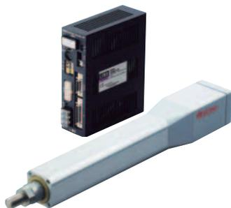
The ball screw is rotated by an  $\alpha$ STEP motor to position even heavy loads with high accuracy. Integrating a motor with a linear motion mechanism, this type of actuator is ideal for applications where the load is pushed or pulled.
