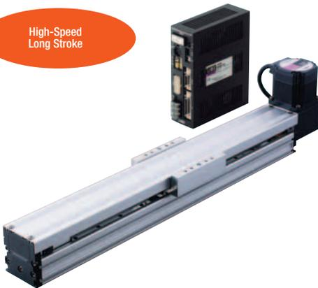
By employing an aluminum frame structure and a belt-and-pulley mechanism, the **SPV6** and **SPV8** support long strokes up to 1000 mm and 1500 mm respectively.
