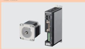
The **RBK** Series is a motor and driver package consisting of a 1.8° step angle stepper motor and DC input microstep driver with a wide input DC voltage range (20 to 75 VDC) and up to 4.5 A/phase (6.3 A/phase peak).
