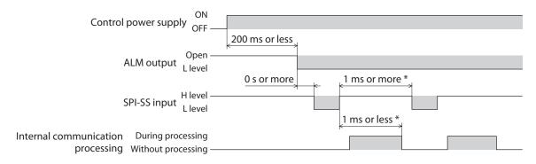
\* When the driver confirms the SPI-SS input has turned from H-level to L-level, it starts processing the received data. Since SPI communication cannot be sent and received while the driver processes the received data, be sure to provide an interval of the communication frame of 1 ms or more.
