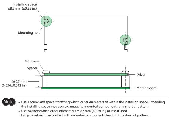
• Provide 9±0.3 mm (0.354±0.012 in.) for the distance between the driver and the motherboard. Failure to do so may cause the CN1 and CN2 connectors to float, leading to contact failure.
