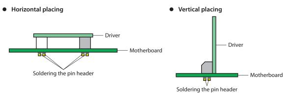
When soldering, do not exceed the following conditions. Soldering by a reflow furnace is not available.
