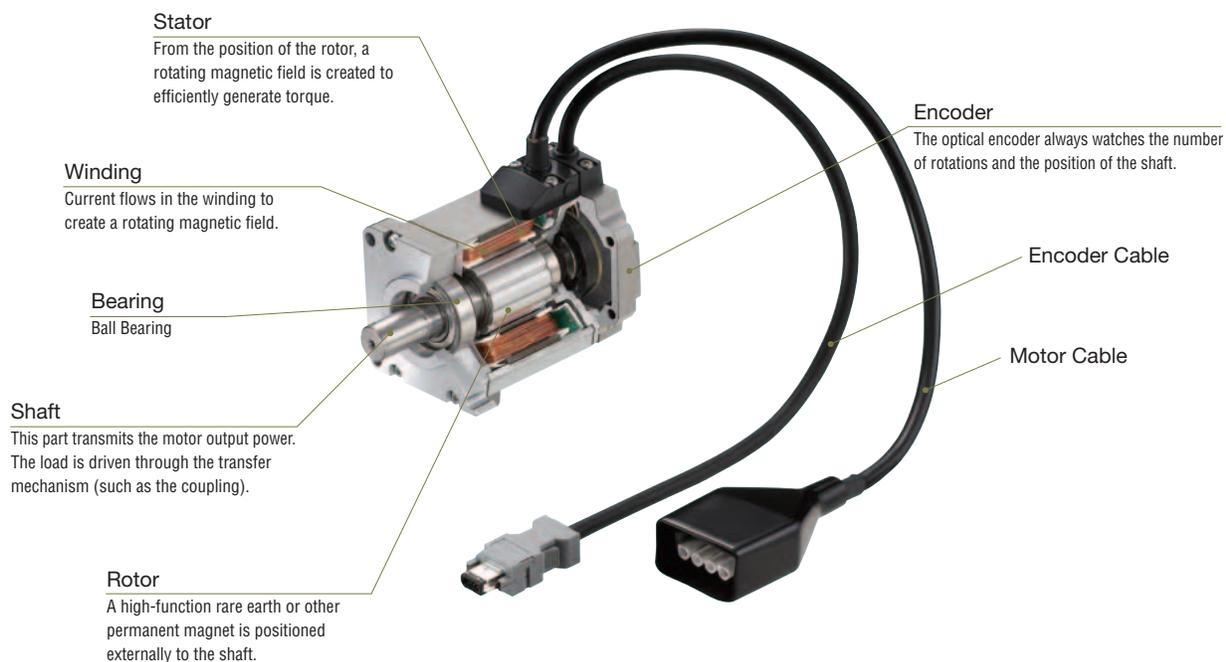
The encoder is a sensor for detecting the speed and position of the motor.
