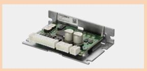
This is a DC power supply input driver for stepper motors. A bipolar driver for 2-phase stepper motors and a driver for 5-phase stepper motors are available.
