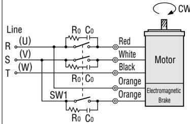
SW1 operates both motor and electromagnetic brake action. The motor will rotate when SW1 is switched simultaneously to ON (short circuit). When SW1 is switched simultaneously to OFF (open), the motor stops immediately with the electromagnetic brake and holds the load.
