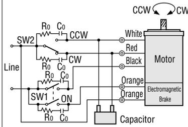
SW1 operates both motor and electromagnetic brake action. The motor will rotate when SW1 is switched simultaneously to ON (short circuit). When SW1 is switched simultaneously to OFF (open), the motor stops immediately with the electromagnetic brake and holds the load.
