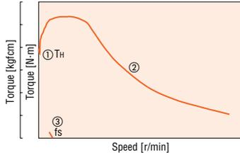
The speed-torque characteristics are determined by the motor and driver, so they vary greatly based upon the type of the driver used.
