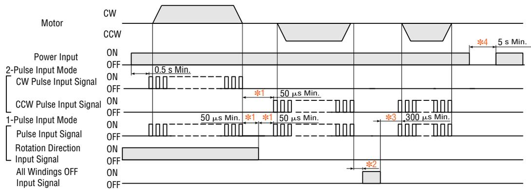
\*1 Switching time to change CW, CCW pulse (2-pulse input mode)
