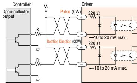
The characters indicate signals under the 1-pulse input mode, while the characters in parentheses indicate signals under the 2-pulse input mode.
