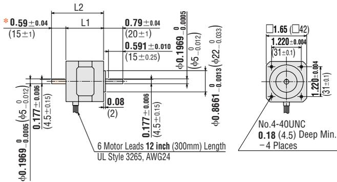
\* The length of machining on double shaft model is  $0.591 \pm 0.010$  (15 ± 0.25).
