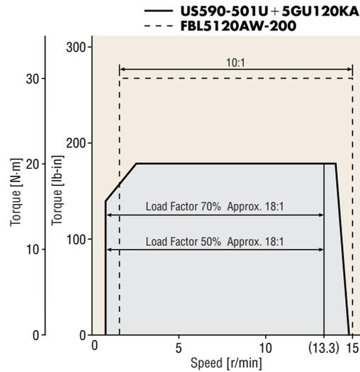
The maximum permissible torque of the **5GU120KA**, which has a gear ratio of 120:1, is 177 lb-in (20 N·m). The speed ratios at 50% and 70% load factors are shown in the table below:
