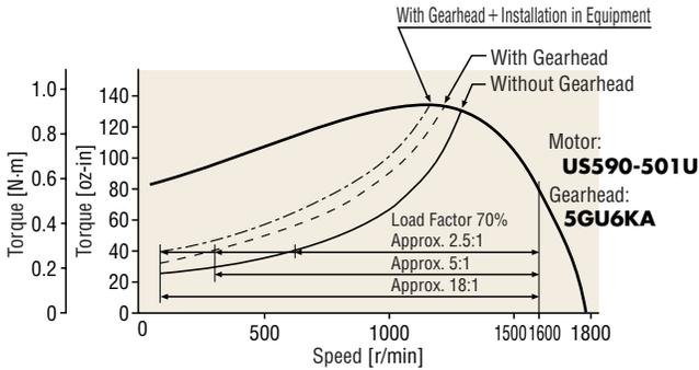
Due to the aforementioned advantage of heat dissipation, when a motor is installed in equipment it can often be operated at variable speeds with a speed ratio of 18:1, as long as the load factor does not exceed 70%.
