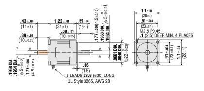
PMC35A3 (Single shaft) Motor Model : PMM35A2 Weight 0.38 lb. (Mass 0.17kg) PMC35B3 (Double shaft) Motor Model : PMM35B2 Weight 0.38 lb. (Mass 0.17kg)
