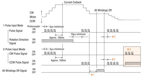
inputting the "All Windings Off" signal to allow the motor oscillations to end. This time varies with the load inertia, the load torque and the starting pulse rate. Do not input the "All Windings Off" signal before the motor has stopped.
