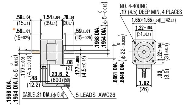
\*.59±.01(15±0.25) indicates the length of milling on motor shaft.
