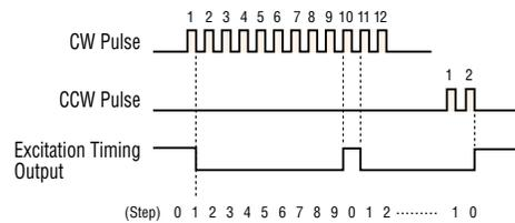
When using the "Excitation Timing" signal, set the number of input pulses and the step angle in combinations which allow the motor shaft to stop at positions which are multiples of 7.2°.
