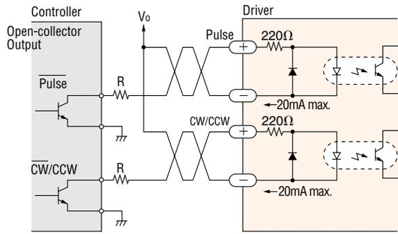
Keep the voltage between DC 5V and DC 24V.
