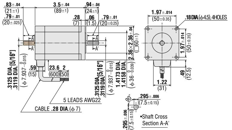
\*.59±.01(15±0.25) indicates the length of milling on motor shaft.
