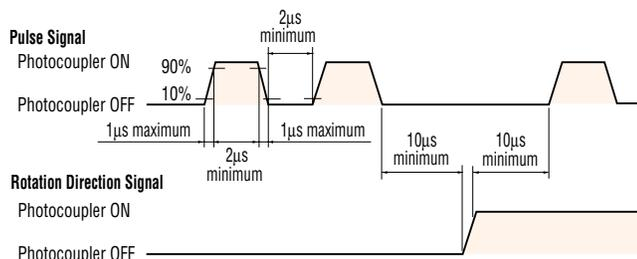
The shaded area indicates when the photocoupler diode is ON. The motor moves when the photocoupler state changes from ON to OFF as indicated by the arrow.
