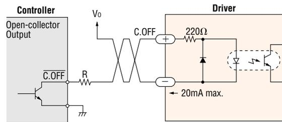
Keep the voltage between DC 5V and DC 24V. When voltage is equal to DC 5V, external resistance (R) is not necessary. When voltage is above DC 5V, connect external resistance (R) and keep the input current below 20mA.
