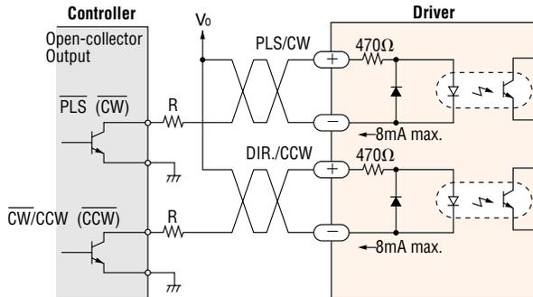
Keep the voltage between DC 5V and DC 12V.
