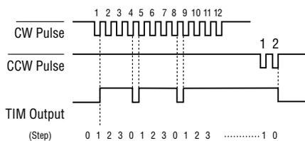
When used as indicated in the sample connection, the level becomes "L" at STEP 0.
