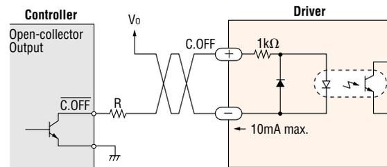
Keep the voltage between DC 5V and DC 12V.
