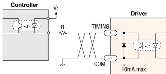
Keep the voltage between DC 5V and DC 30V.
