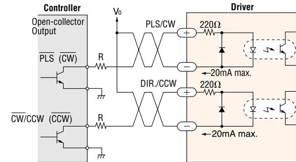
Keep the voltage between DC 5V and DC 24V. When voltage is equal to DC 5V, external resistance (R) is not necessary. When voltage is above DC 5V, connect external resistance (R) and keep the input current below 20mA.
