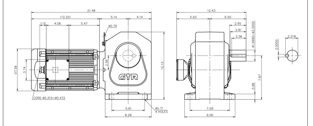
NOTE: THE RATING OF ENCLOSURE CLASS: IP65 (EN60034-5) EQUIVALENT.
