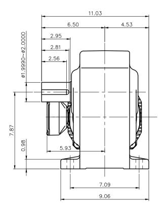
NOTE: THE RATING OF ENCLOSURE CLASS: IP65 (EN60034-5) EQUIVALENT.
