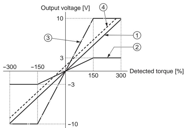
**Note** Even when a torque above the maximum voltage is detected, the output will not exceed the maximum voltage.
