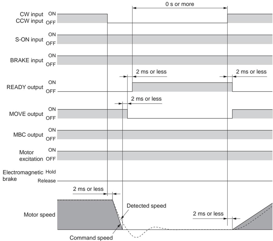
■ CW input/CCW input [torque control mode, tension control mode]
