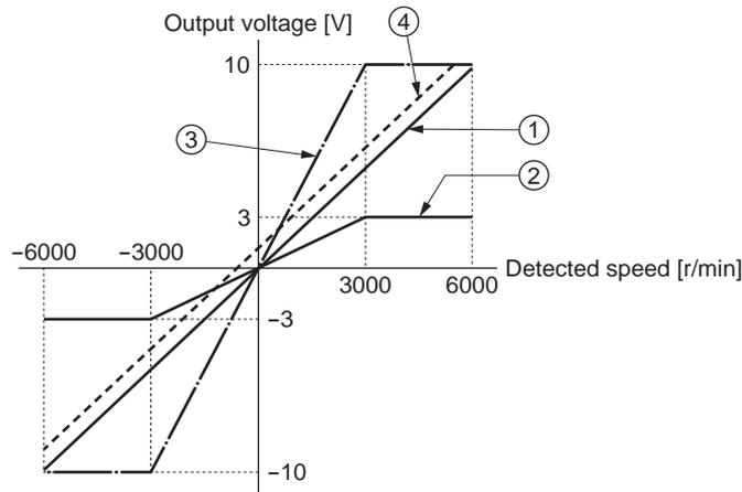
**Note** Even when a speed above the maximum voltage is detected, the output will not exceed the maximum voltage.
