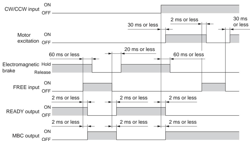
When the parameter for operation selection after stopping in speed control mode [SyS-1-02] is set to “Servo lock”
