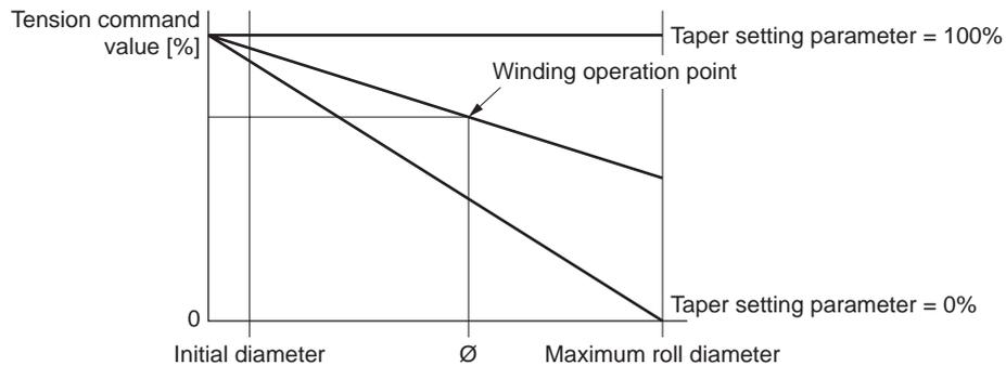
When the roll diameter is "0," the tension command value is used. Once the roll diameter reaches the maximum diameter, the taper setting will be applied to the tension command value.
