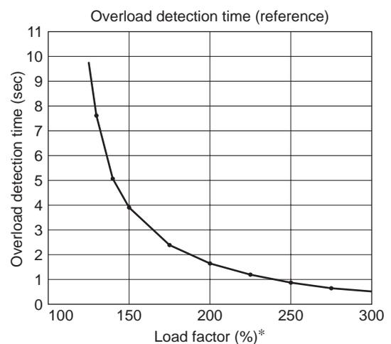
\* The load factor is 100% when the rated torque is output.
