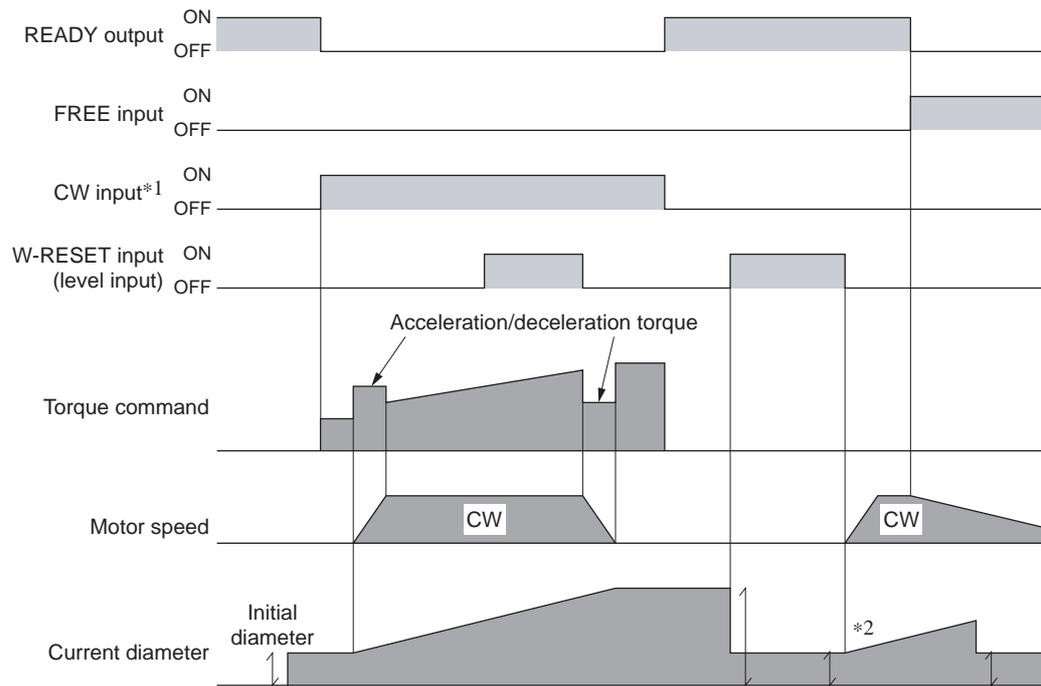
\*1 In high function mode I and high function mode II, the CCW input is disabled.
