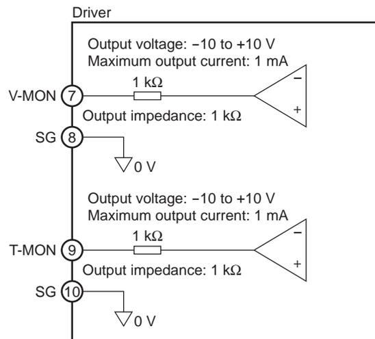
**Note** The output impedance is 1 kΩ. Check the input impedance of the measuring instrument or external circuit to be connected.
