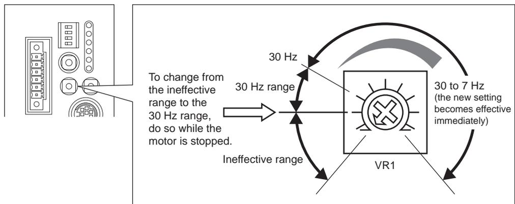
**Note** To change the damping control frequency from the ineffective range to the 30 Hz range, stop the motor before turning the VR1. Changing the setting while the motor is operating may cause the motor to move the equipment abruptly.
