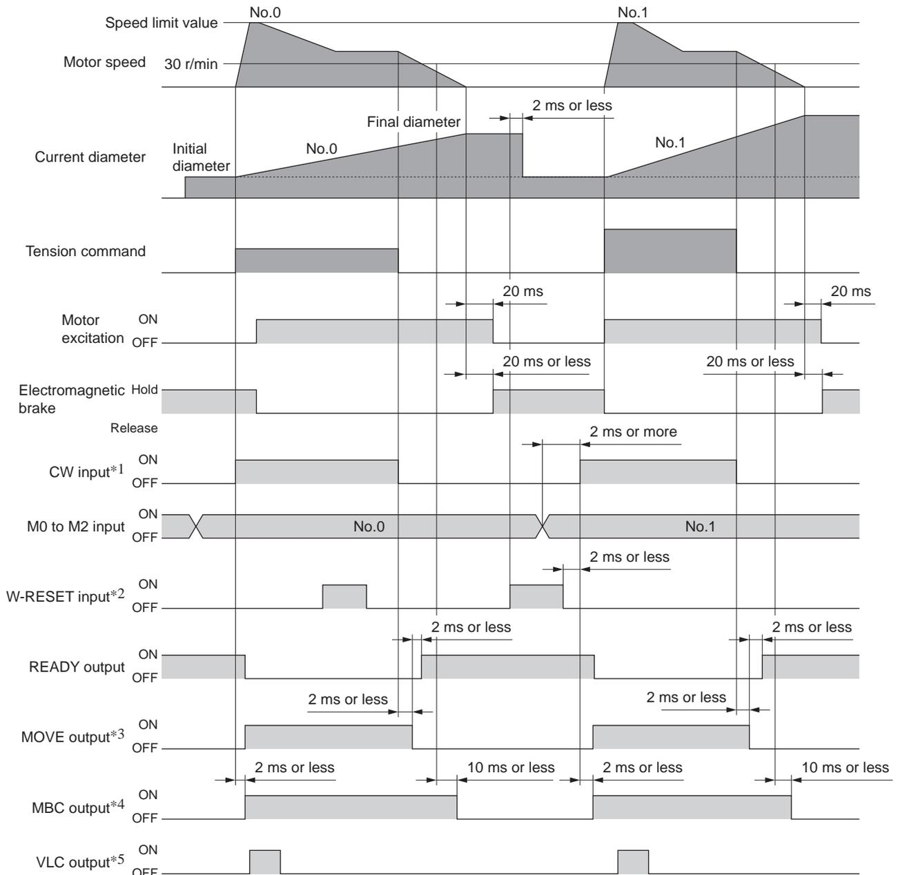
\*1 The direction in which the motor rotates when the CW input turns ON can be set in the system parameter for motor rotation direction [SyS-1-06].
