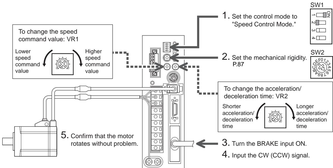
**Note** The new settings of the control mode setting switches will become effective after the power is cycled. If a 24 VDC power supply is used, also cycle the 24 VDC power supply.
