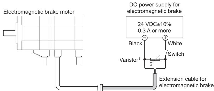
\* To protect the switch contacts and prevent noise, the customer is advised to provide a varistor [recommended varistor: Z15D121 (Ishizuka Electronics Corporation)].
