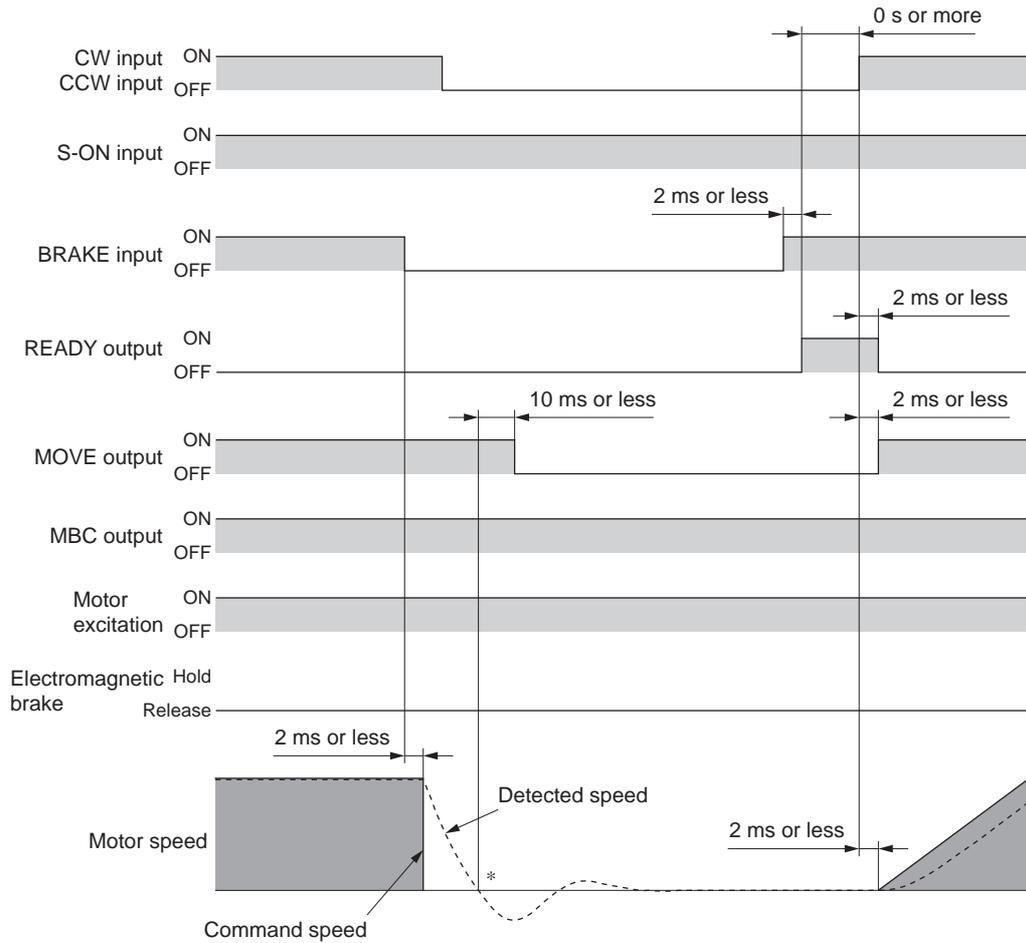
\* The MOVE output will turn OFF when the detected speed becomes zero.
