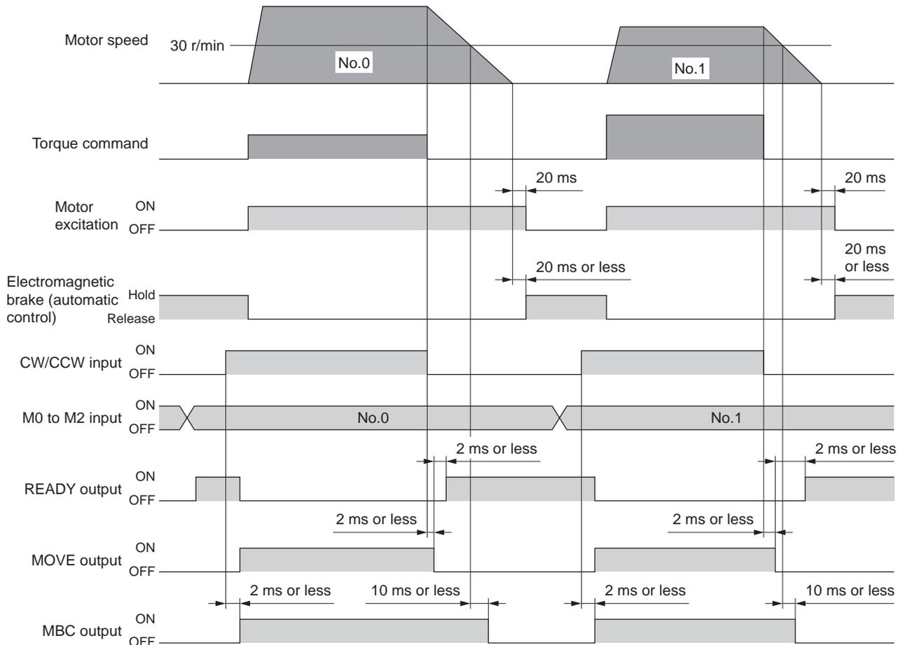
\* When the CW (or CCW) input is turned OFF, the motor will remain excited for approx. 20 ms after the torque command is completed.
