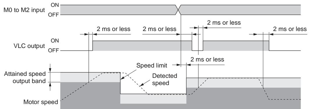
■ ZV output [speed control mode, torque control mode, tension control mode]
