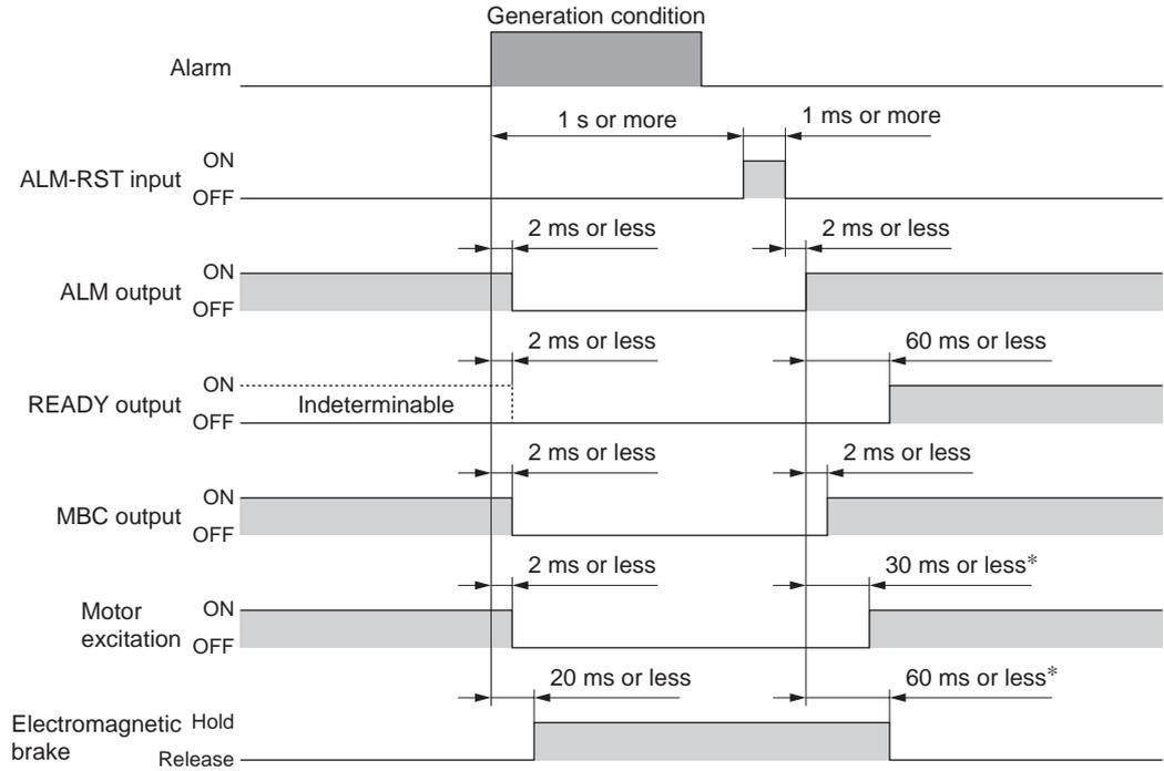
\* In the position control mode or speed control mode (servo locked upon stopping) when the S-ON input is ON. In the torque control mode and tension control mode, the motor will remain unexcited and the electromagnetic brake will continue to hold the load in position until a start signal is input.
