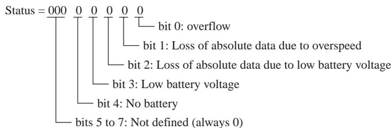
Example: When an overflow alarm has generated
