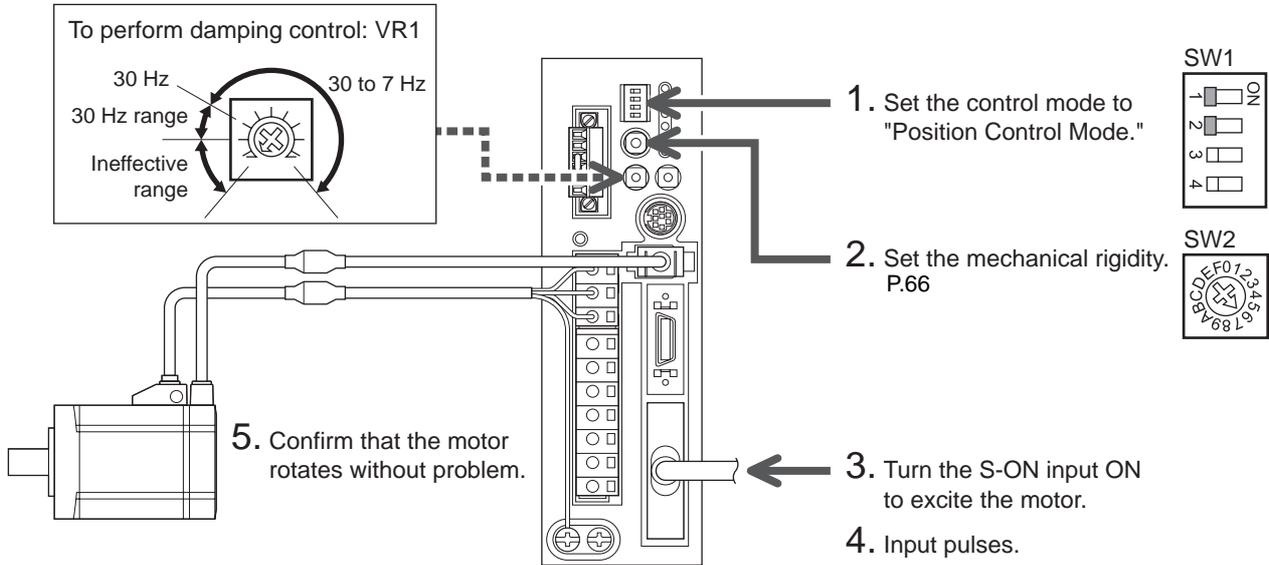
**Note** The new settings of the control mode setting switches will become effective after the power is cycled. If a 24 VDC power supply is used, also cycle the 24 VDC power supply.
