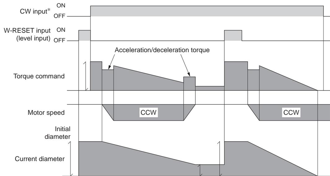
The current diameter is clipped when the roll diameter becomes zero.
