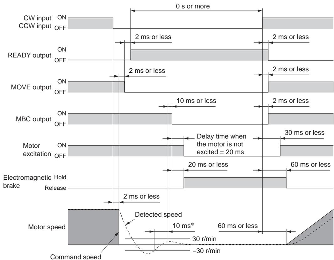
\* If the detected speed remains at or below  $\pm 30$  r/min for 10 ms or more, the MBC output will turn OFF.
