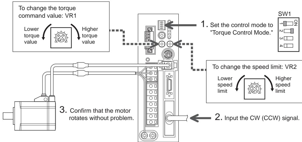
**Note** The new settings of the control mode setting switches will become effective after the power is cycled. If a 24 VDC power supply is used, also cycle the 24 VDC power supply.
