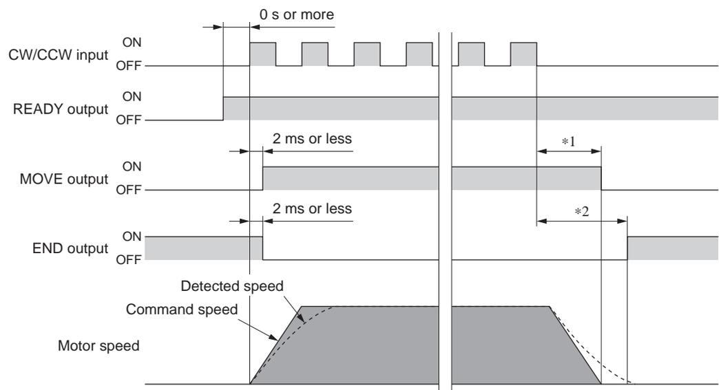
\*1 The specific time varies depending on the setting of the application parameter for command filter [APP-4-01].
