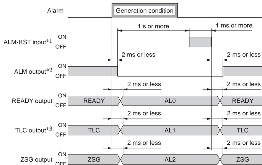
\*1 An alarm is reset at the ON→OFF edge. Before resetting an alarm, be sure to remove the cause of the alarm, and then input the signal only once.
