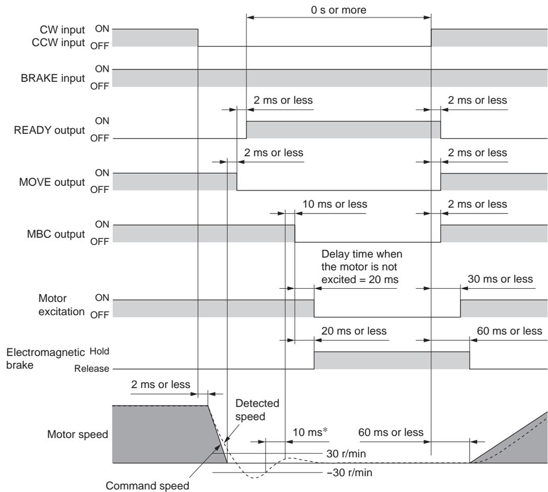
\* If the detected speed remains at or below  $\pm 30$  r/min for 10 ms or more, the MBC output will turn OFF.
