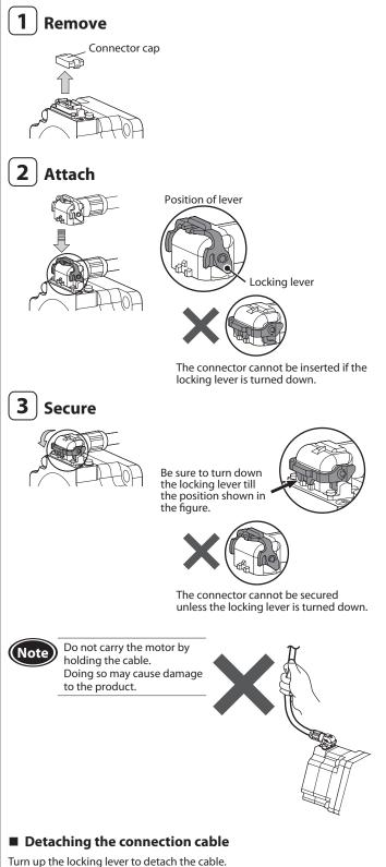
The connection cable for relay can be used by connecting up to 2 pieces. Check the operating manual supplied with the driver.
