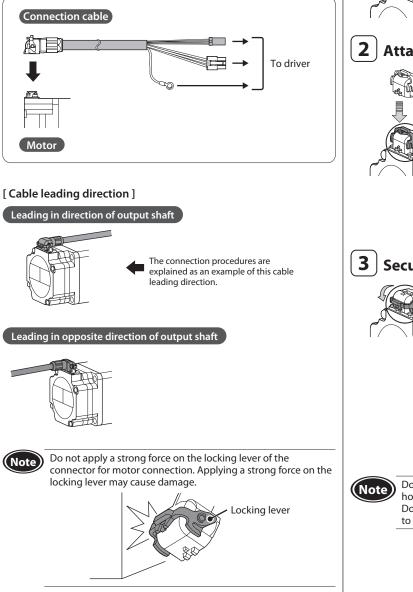
Connection procedures of the motor and connection cable
