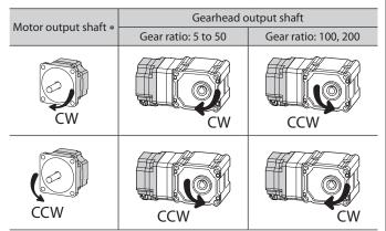
\* Check the operating manual supplied with the driver for the rotation direction of the motor output shaft and the setting method.
