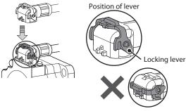
The connector cannot be inserted if the locking lever is turned down.
