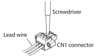
3. Insert the CN1 connector into power supply connector (CN1) and tighten the screws using a screwdriver (connector screw size: M2.5).
