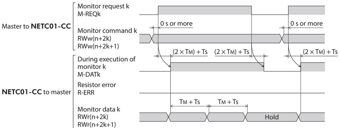
$T_M$ : Communication time between the CC-Link communication master station and remote device station (NETC01-CC) [Check the operating manual of the master station.]
