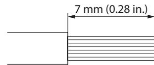
2. Insert each lead wire into the CN1 connector and tighten the screw using a screwdriver (connector screw size: M2).
