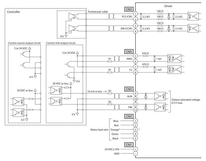
\* This orange lead wire is for 5-phase stepping motor. For 2-phase stepping motor, do not connect anything to the pin No.3 since there is no orange lead wire.
