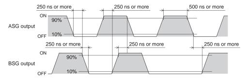
The electrical characteristics vary depending on the IC specification of the line driver.
