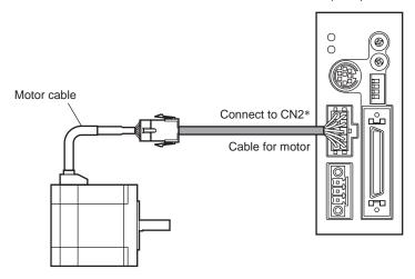
$^{*}$  Keep 30 m (98.4 ft.) or less for the wiring distance between the motor and driver.
