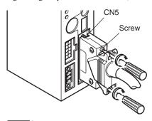
Note Be certain the I/O signals cable is as short as possible. The maximum input frequency will decrease as the cable length increases.
