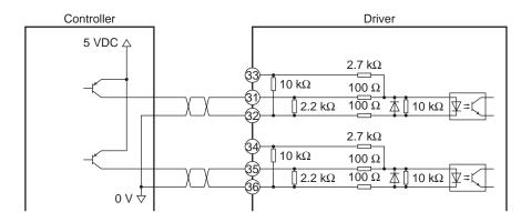
• When pulse input is of 24 VDC type
