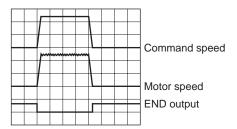
• Speed filter setting switch=F (maximum)
