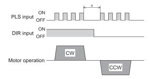
\* The minimum interval time needed for switching the direction of rotation will vary, depending on the operating speed and size of the load. Do not shorten the interval time more than necessary.
