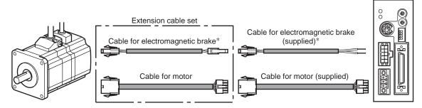
\* Only when the motor is of electromagnetic brake type.
