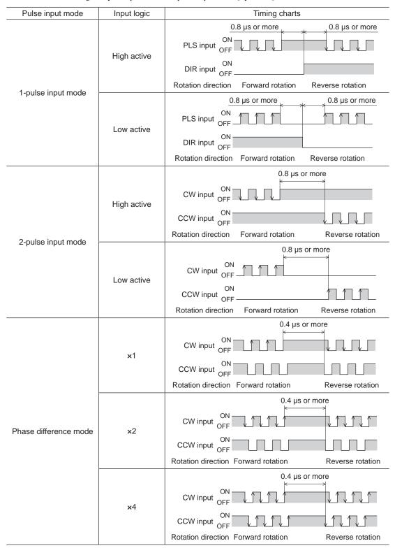
Whether to cause the motor to rotate in CW direction or CCW direction when a forward direction pulse is input can be set using the system parameter for rotation direction [SyS-1-04]. Refer to page 47.
