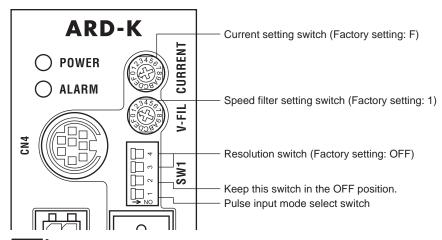
Note Before operating any switch, turn off the driver power and wait for the POWER LED to turn off.
