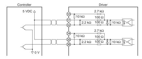
• When pulse input is of 24 VDC type
