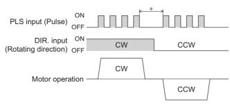
\* The minimum interval time needed for switching the direction of rotation will vary, depending on the operating speed and size of the load. Do not shorten the interval time any more than is necessary.
