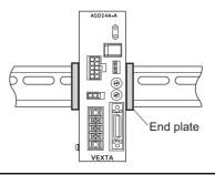
• Removing from DIN rail
