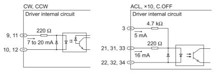
The same voltage must be set for the following two voltages. Connecting both 5 and 24 VDC power supplies may damage the driver and power supplies. • Voltage for ACL input, ×10 input and C. OFF input (Pin Nos. 21, 22, 31, 32, 33 and 34) • Voltage for TIM.1/TIM.2 outputs, ASG1/ASG2 outputs and BSG1/BSG2 outputs (Pin Nos. 1 and 2)
