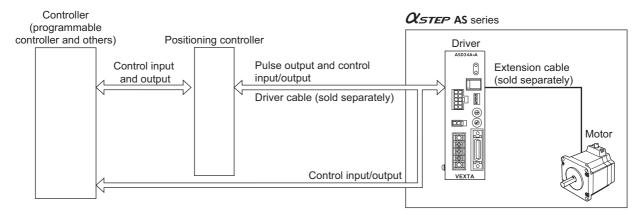
• Extension cables are available in two types: the standard type and the electromagnetic brake type. If you are using an electromagnetic brake motor, provide a 24 VDC power supply for the electromagnetic brake separately from the control power supply and always use an optional extension cable of the electromagnetic brake type (sold separately) for connection. The electromagnetic brake will not function if the motor cable is connected directly to the driver.
