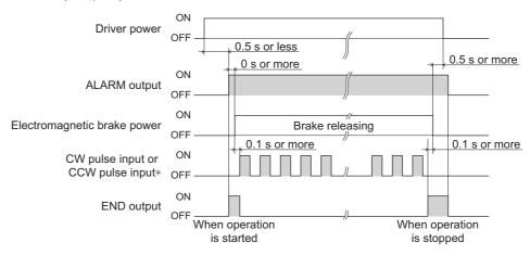
\* CCW input is enabled when 2-pulse input mode is selected
