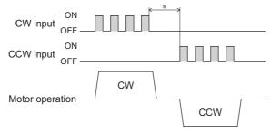
\* The minimum interval time needed for switching the direction of rotation will vary, depending on the operating speed and size of the load. Do not shorten the interval time any more than is necessary.
