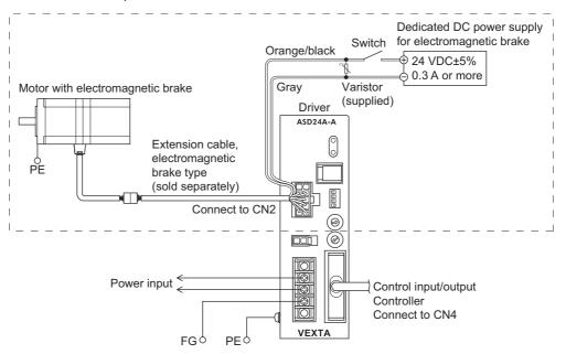
The colors of the two lead wires (orange and gray) extending from the driver's connector side of the flexible extension cable of the electromagnetic brake type differ from those of the extension cable.
