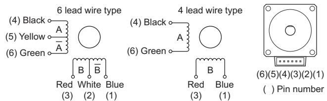
The colors of lead wires shown apply to the supplied connection cable or optional connection cable. If you are using the connector set or when you are providing your own connector or lead wire, connect based on the pin numbers shown.
