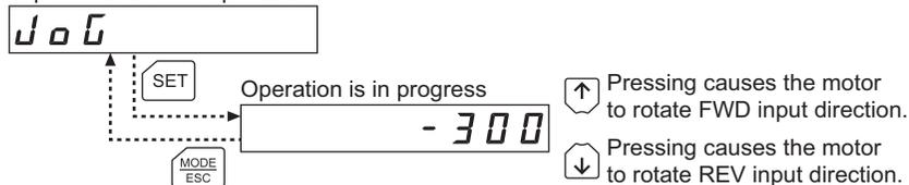
**Note** During JOG operation, the motor rotates at the specified operation speed while each applicable key is pressed. Before commencing JOG operation, consider the status of the equipment and condition of its surroundings to confirm thoroughly that motor rotation will not cause any dangerous situation.
