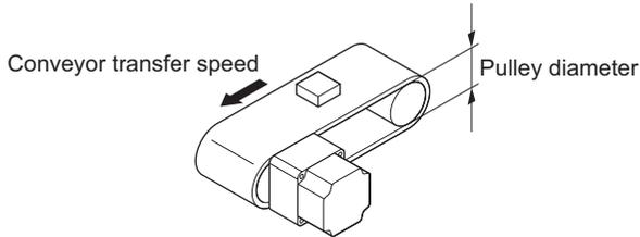
When the calculated conveyor speed reduction ratio is used, the conveyor transfer speed is converted as follows:
