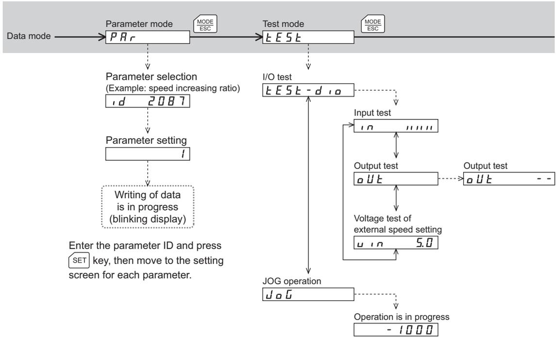
Enter the parameter ID and press **SET** key, then move to the setting screen for each parameter.
