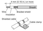
To ground a shielded cable, use a metal that will maintain contact with the entire circumference of the cable. Attach a cable clamp as close to the end of the cable as possible, and connect it as shown in the figure.
