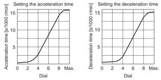
\* However, when the load inertia is large, the deceleration time cannot be set at a shorter time than how long it takes for the motor to coast to a stop.
