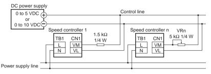
Current capacity (I) of external DC power supply when the number of speed controllers is n: Current capacity (I) =  $1 \times n$  (mA)
