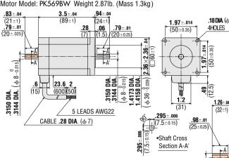
.5512 DIA. .5505 DIA. ( •These external appearance drawings are for double shaft models For a single shaft, ignore the colored areas.
