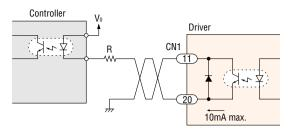
Keep the voltage between DC 5V and DC 24V.
