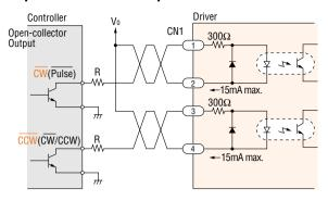
Keep the voltage between DC 5V and DC 24V.
