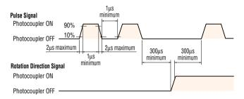
The shaded area indicates when the photocoupler is ON. The motor moves when the photocoupler state changes from ON to OFF as indicated by the arrow.
