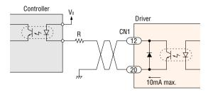
Keep the voltage between DC 5V and DC 24V. Keep the current below 10mA. If the current exceeds 10mA, connect external resistance (R).
