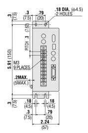
•I/O Signal Connector (Included) Connector: 54306-2011 (MOLEX) Connector Cover: 54331-1201 (MOLEX)
