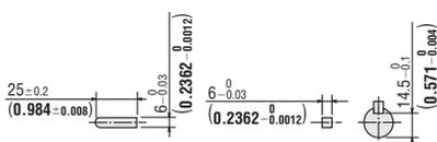
● At the time of shipment, a key is inserted on the gearhead's shaft.
