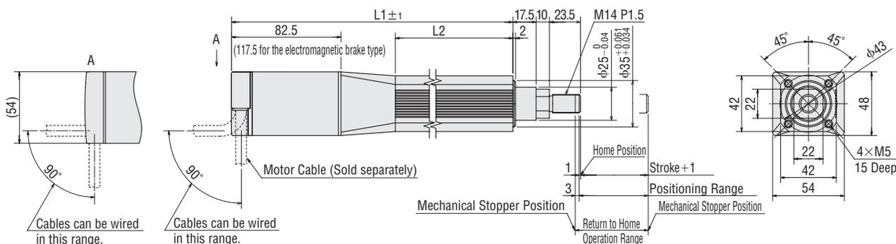
Cylinder Model: EZC4D□A, EZC4E□A, EZC4D□C, EZC4E□C (Without electromagnetic brake)
