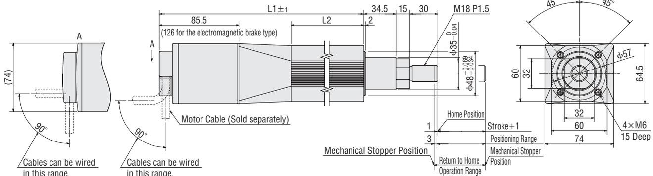
Cylinder Model: EZC6D□K, EZC6E□K (Without electromagnetic brake)
