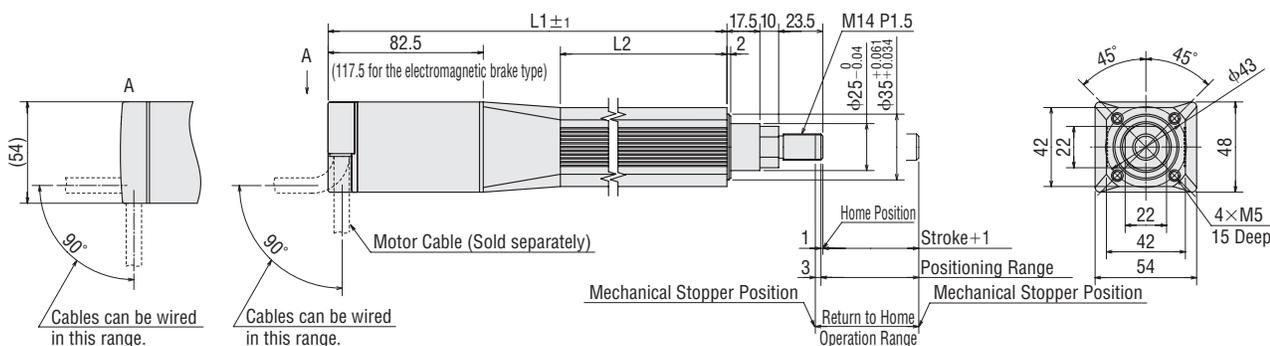
Cylinder Model: EZCM4D□K, EZCM4E□K (Without electromagnetic brake)
