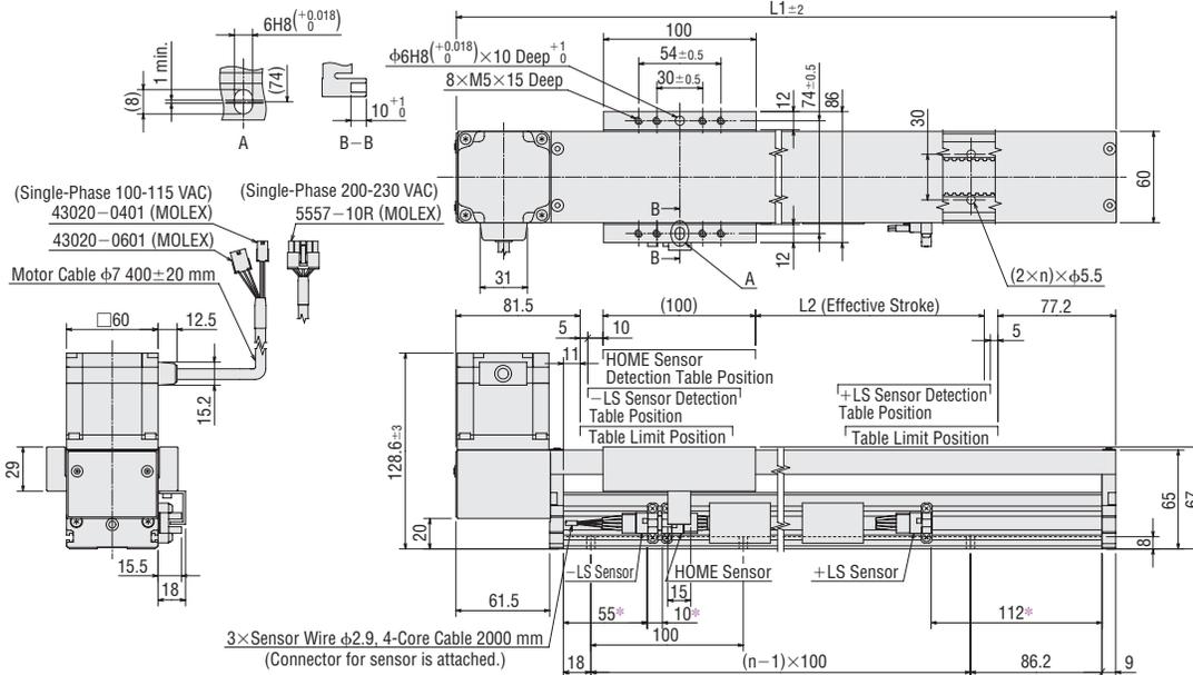
\* The settings "55," "10" and "112" indicate the recommended mounting positions of the -LS sensor, HOME sensor and +LS sensor, respectively. Sensors and a shield plate can also be installed on the opposite side.
