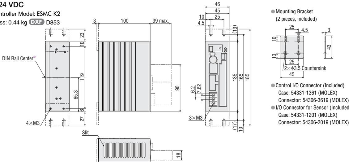
\*The center of the DIN rail when a DIN rail mounting plate (**PADP01**, sold separately) is used for installation.
