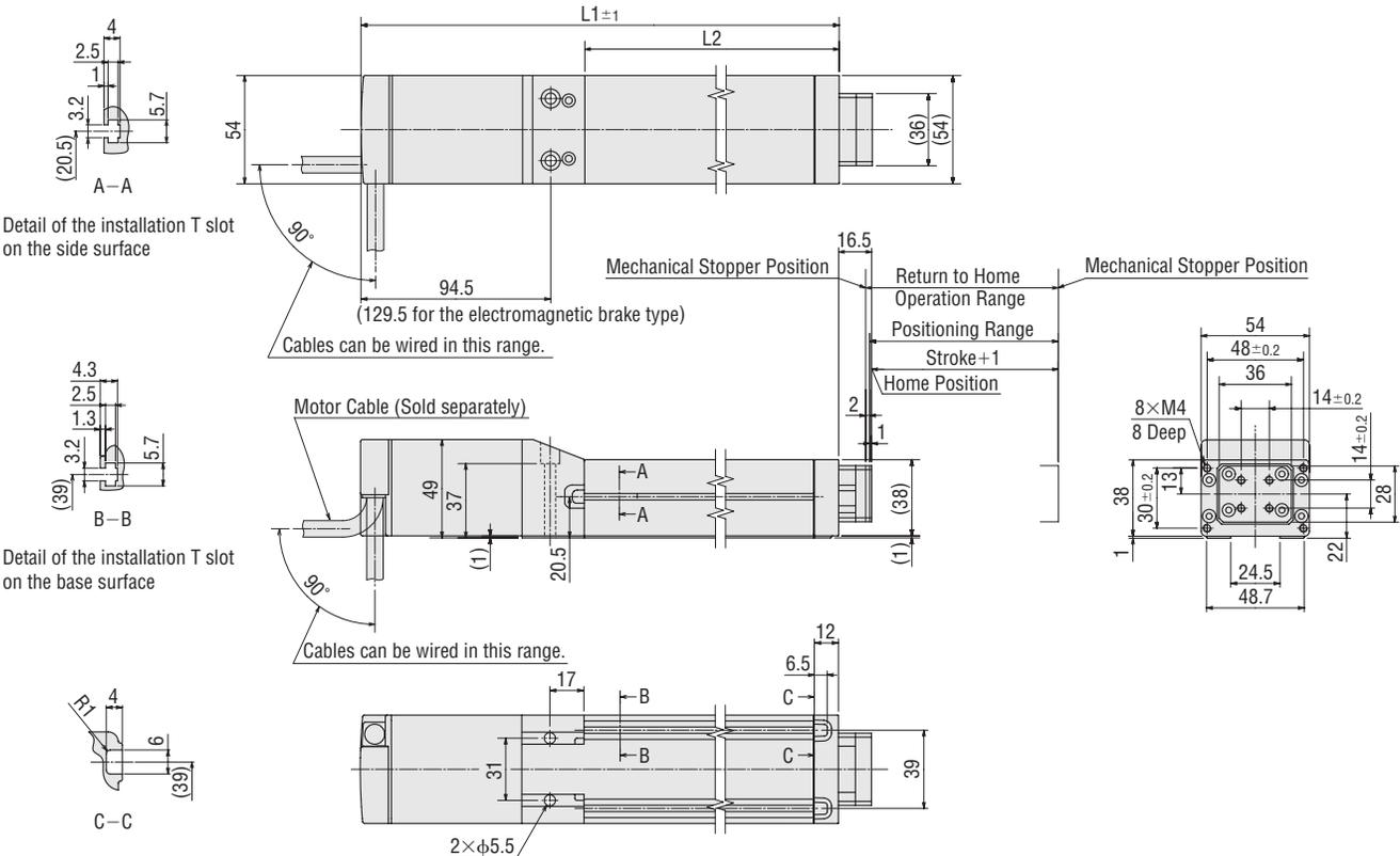
Cylinder Model: EZAM4D□K, EZAM4E□K (Without electromagnetic brake)
