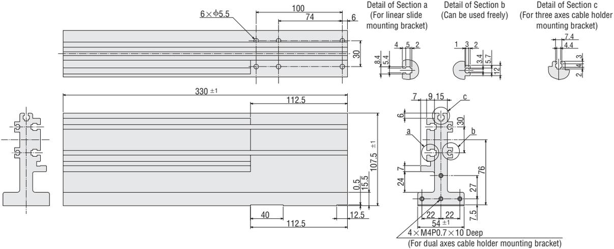
Three Axes Cable Holder Mounting Bracket (1 piece)
