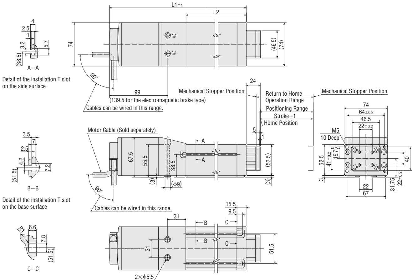
Cylinder Model: EZAM6D□A, EZAM6E□A, EZAM6D□C, EZAM6E□C (Without electromagnetic brake)
