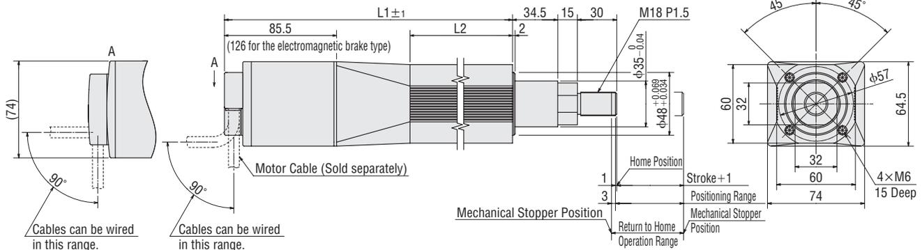
Cylinder Model: EZC6D□A, EZC6E□A, EZC6D□C, EZC6E□C (Without electromagnetic brake)
