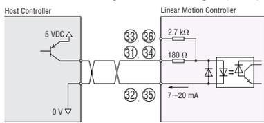
When connecting to a line driver output circuit
