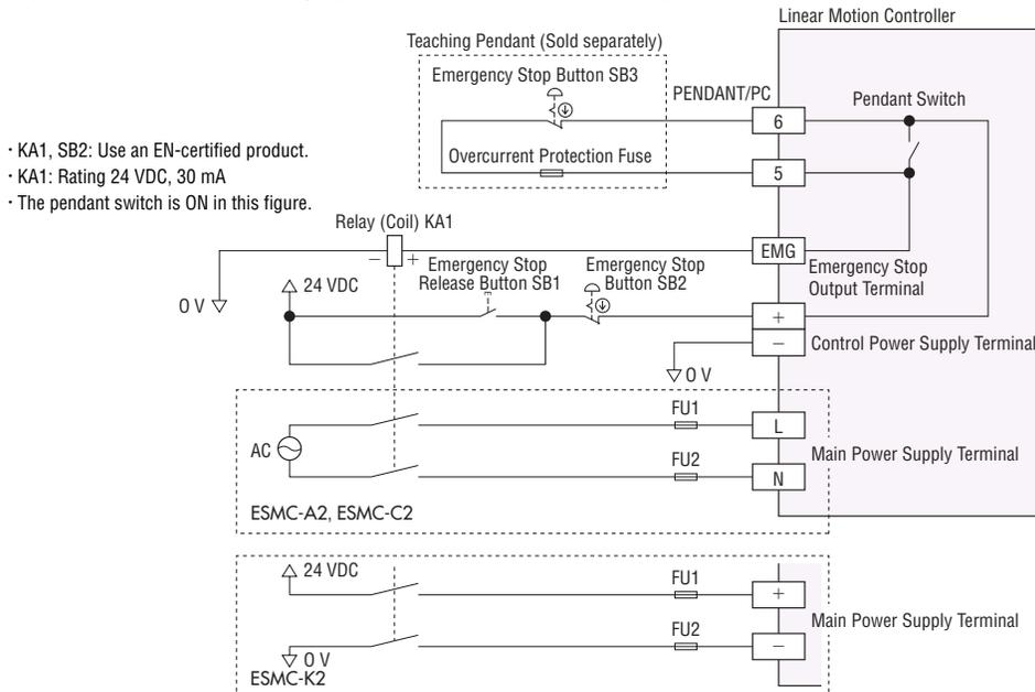
◇ Connection Example When an Emergency Stop Function is Not Used
