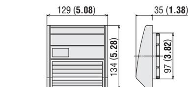
● Dimensions of panel cut-out are also same as those of fan and filter panels.
