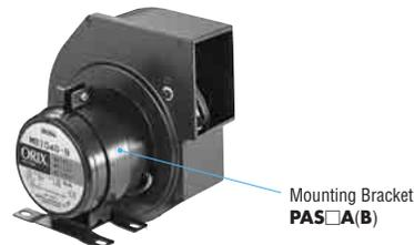
For all the centrifugal blowers except for **MB520** and **MB630**,  $h_2$  is longer than  $h_1$ , therefore, a pedestal must be used when mounting the centrifugal blower so that the casing does not touch the mounting surface. (For exact dimensions, refer to dimensions in each page where product is listed.)
