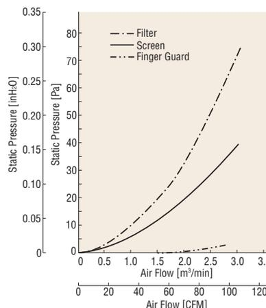
Fig. 10 Pressure Loss Caused by Accessories
