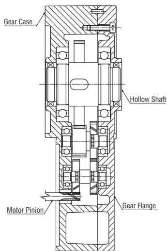
Structure of the Hollow Shaft Flat Gearhead
