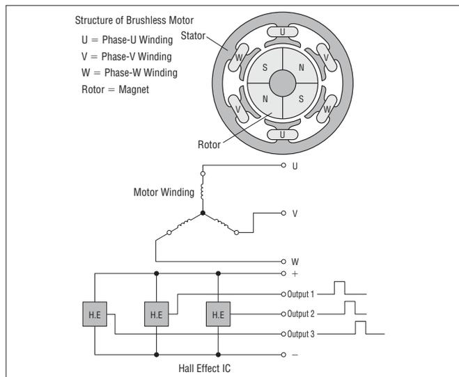
A Hall effect IC is used for the sensor's magnetic element. Three Hall effect ICs are placed within the stator, and send digital signals as the motor rotates.
