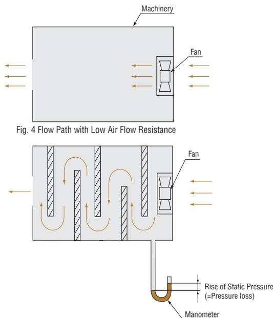
Fig. 4 Flow Path with Low Air Flow Resistance
