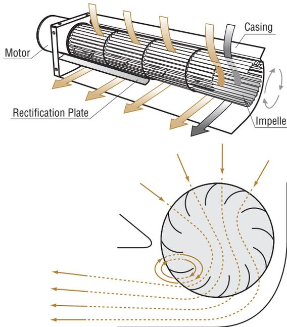
Fig. 3 Structure and Air Flow Mechanism of Cross Flow Fans
