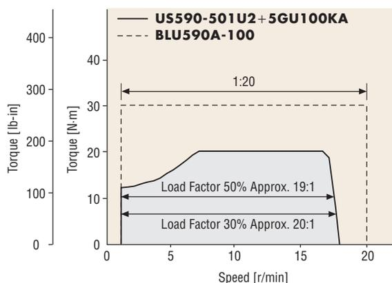
The maximum permissible torque of the **5GU100KA**, which has a gear ratio of 100:1, is 20 N·m (177 lb-in). The speed ratios at load factors of 30% and 50% are shown in the table below:
