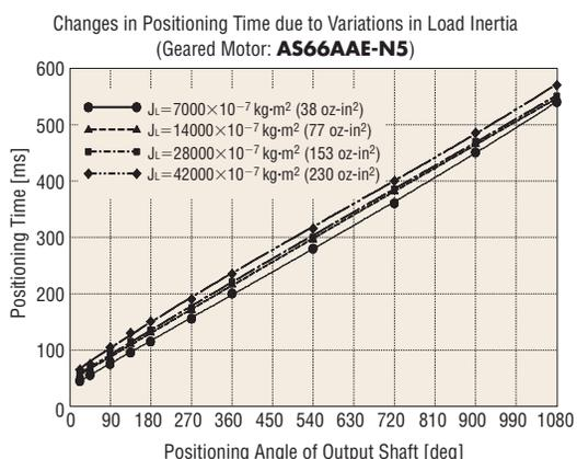
While the shortest positioning time of the standard type motor changes significantly with the increase in inertial load, that of the geared motor shows little change. In other words, the geared motor is capable of driving a larger inertial load within the most consistent, shortest positioning time.
