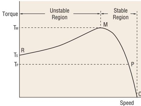
Under no load, the motor rotates at a speed close to synchronous speed. As the load increases, the motor's speed drops to a level (P) where a balance is achieved between load and motor torque ( $T_p$ ). If the load is further increased and reaches point M, the motor can generate no greater torque and stops at point R. In other words, the motor can be operated in a stable range between M and O, while the range between R and M is subject to instability.
