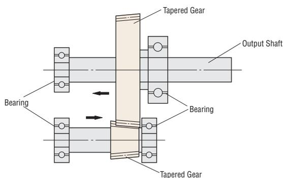
Structure of TH Gear's Final Stage
