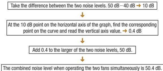
If 40 dB of noise is combined with 50 dB, the resulting increase in noise level is only 0.4 dB. In other words, the noise level is always controlled by the larger of noise values, so it is important to suppress the noise of the fan producing greater noise.
