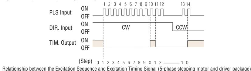
Use these timing signals when it is necessary to perform highly reproducible return to mechanical home operation. The following sections describe stepping motor return to mechanical home operation and the use of timing signals.
