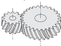
In both types of gearheads, the helical configuration is employed for the motor pinion and its mating gear. This contributes significantly to noise reduction because of their high contact speeds, thereby achieving lower noise output.
