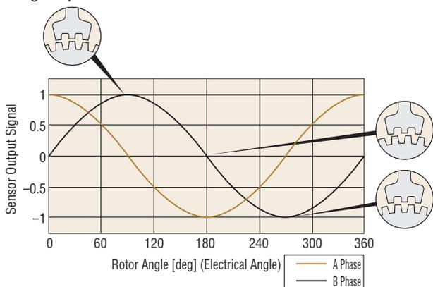
Output Signal of Rotor Position Detection Sensor
