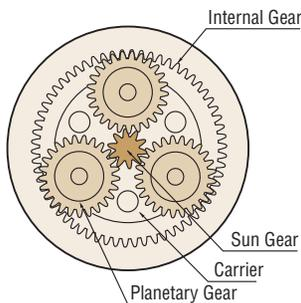
Cross Section of a PN Gear
