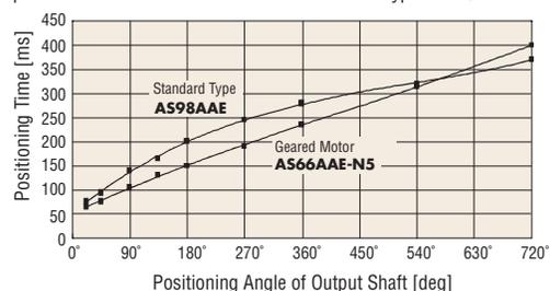
The geared motor is more effective in reducing the positioning time for a smaller positioning angle and a larger inertial load. The geared motor tends to achieve shorter positioning time in a wider range of positioning angles with a larger inertial load.
