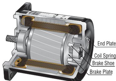
The brake mechanism is constructed as shown in the figure above. The coil spring applies constant pressure to allow the brake shoe to slide toward the brake plate.
