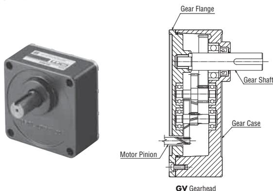
For use with standard AC motors, many of which are constant speed motors, the availability of various gear ratios suits a wide range of desired speeds. We support these motors with 20 different gear ratios, ranging from 3:1 to 180:1.
