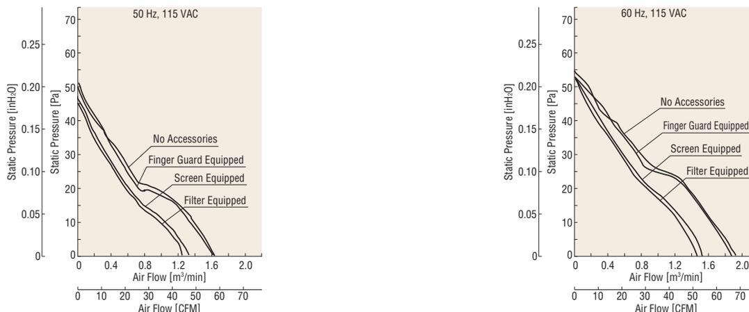
Fig. 11 Changes in Characteristics with Accessories Equipped to the MU1225S-21
