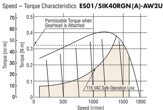
● Safe-Operation Line and Permissible Torque When Gearhead is Attached
