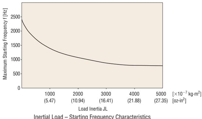
Changes in maximum starting frequency with the inertial load may be approximated via the following formula:
