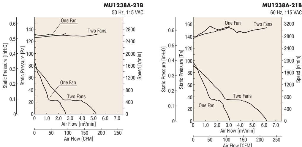
Fig. 9 Changes in Air Flow – Static Pressure Characteristics Using Two Fans
