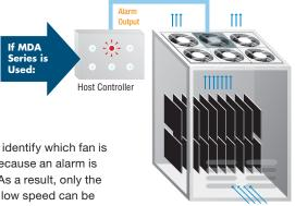
You can identify which fan is failing because an alarm is output. As a result, only the fan with low speed can be replaced.
