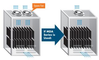
A spare fan is installed in case the cooling capacity decreases.
