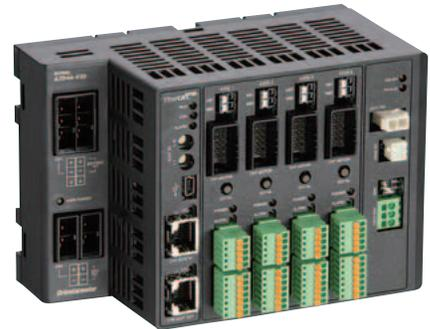
A multi-axis driver that supports EtherCAT communication. Compatible with the CiA402 drive profile. It can be connected to the **AZ** Series DC input motors and electric actuators. 2-axes, 3-axes and 4-axes driver connections are available.
