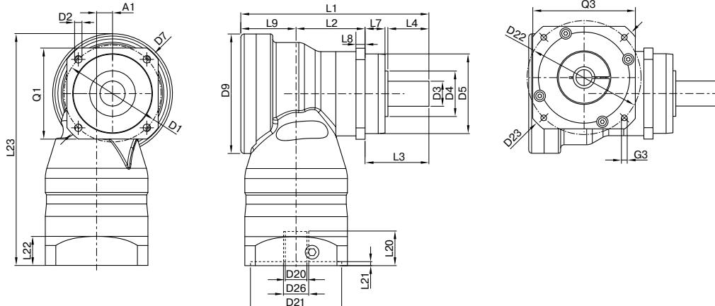
Drawing corresponds to a WPLN090 / 1-stage / smooth output shaft / 19 mm clamping system / motor adaptation – 2-part – round universal flange / B5 flange type motor
