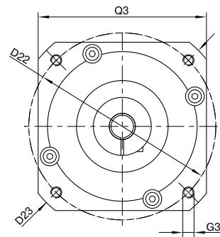
Drawing corresponds to a PSBN090 / 1-stage / smooth output shaft / 14 mm clamping system / motor adaptation – 2-part – round universal flange / B5 flange type motor
