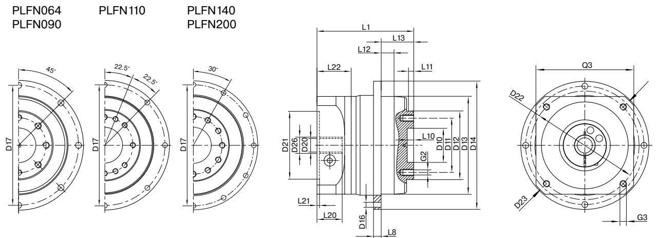
Drawing corresponds to a PLFN090 / 1-stage / flange output shaft / 19 mm clamping system / motor adaptation – 2-part – round universal flange / B5 flange type motor
