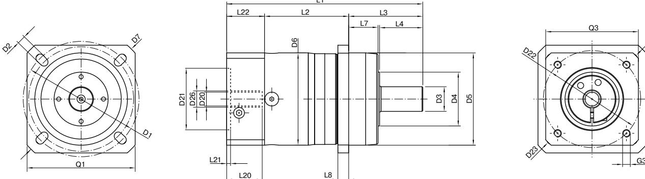
Drawing corresponds to a PLHE060 / 1-stage / smooth output shaft / 11 mm clamping system / motor adaptation – one part / B5 flange type motor
