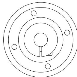
Drawing corresponds to a PLE060 / 1-stage / output shaft with feather key / 11 mm clamping system / no motor adaptation – round universal flange
