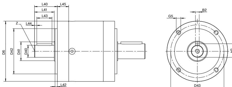
Drawing corresponds to a PLE080 / 1-stage / output shaft with feather key / input shaft – All other variants can be retrieved in Tec Data Finder at [www.neugart.com](http://www.neugart.com)
