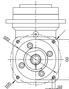
Drawing corresponds to a WPLFE090 / 1-stage / flange output shaft with dowel hole / 19 mm clamping system / motor adaptation – 2-part – square universal flange / B5 flange type motor
