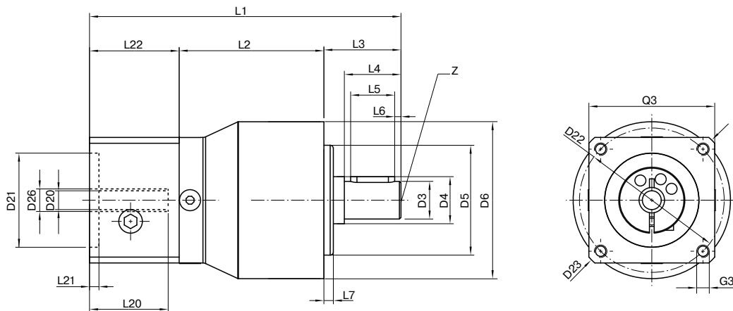
Drawing corresponds to a PLPE050 / 1-stage / output shaft with feather key / 8 mm clamping system / motor adaptation – one part / B5 flange type motor
