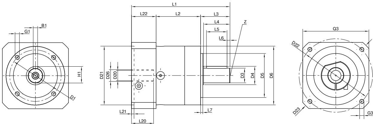
Drawing corresponds to a PLE060 / 1-stage / output shaft with feather key / 11 mm clamping system / motor adaptation – one part / B5 flange type motor
