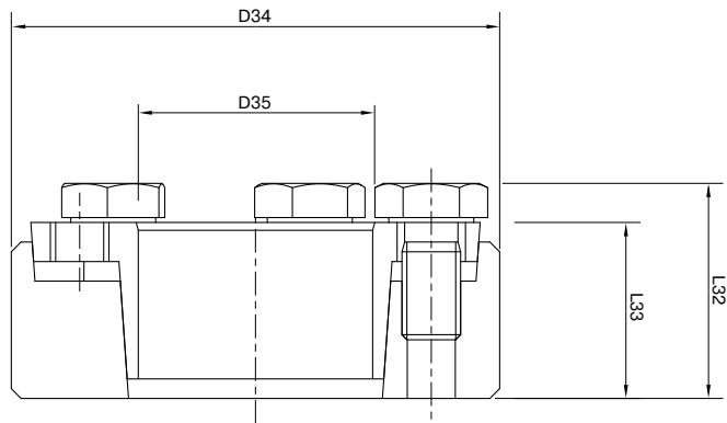
This shrink disc can be used to make a force-fit connection between your machine shaft and the right angle hollow shaft gearbox WGN.
