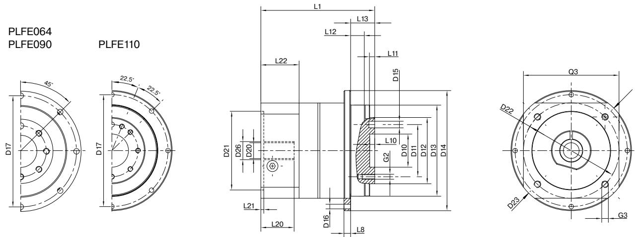
Drawing corresponds to a PLFE110 / 1-stage / flange output shaft with dowel hole / 24 mm clamping system / motor adaptation – one part / B5 flange type motor
