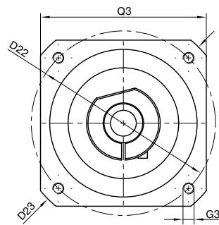
Drawing corresponds to a PLQE080 / 1-stage / output shaft with feather key / 19 mm clamping system / motor adaptation – one part / B5 flange type motor
