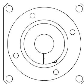
Drawing corresponds to a PLE060 / 1-stage / output shaft with feather key / 19 mm clamping system / no motor adaptation – square universal flange
