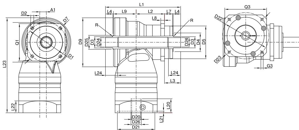
Drawing corresponds to a WGN090 / 1-stage / hollow output shaft on both sides / 19 mm clamping system / motor adaptation – 2-part – round universal flange / B5 flange type motor
