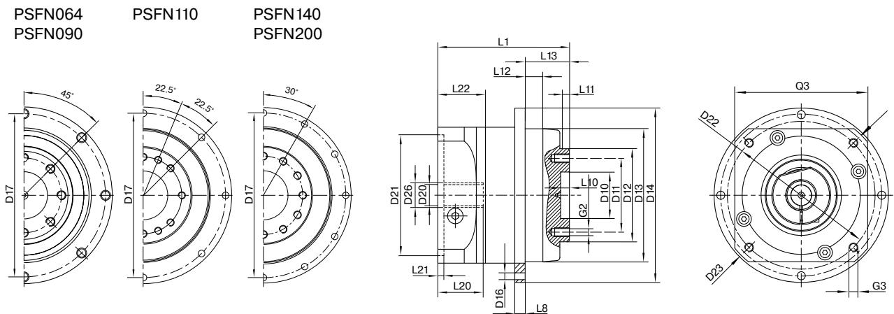
Drawing corresponds to a PSFN090 / 1-stage / flange output shaft / 14 mm clamping system / motor adaptation – 2-part – round universal flange / B5 flange type motor
