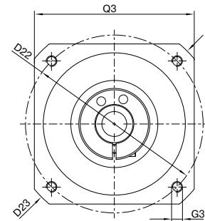
Drawing corresponds to a PLN090 / 1-stage / smooth output shaft / 19 mm clamping system / motor adaptation – 2-part – round universal flange / B5 flange type motor
