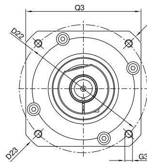
Drawing corresponds to a PSN090 / 1-stage / smooth output shaft / 14 mm clamping system / motor adaptation – 2-part – round universal flange / B5 flange type motor
