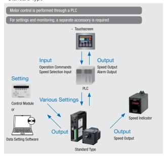
• The motor is controlled through inputs received from a switch box, PLC, or the like. Motor speed, alarm, and other signals are output to the master control system.
