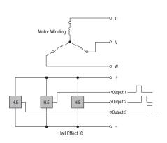
A hall effect IC is used for the sensor's magnetic component. 3 hall effect ICs are placed within the stator and output digital signals as the rotor rotates.
