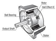
The brushless motor has a built-in magnetic component or optical encoder for the detection of rotor position. The position detectors send signals to the drive circuit. The brushless motor uses three-phase windings in a "star" connection. A permanent magnet is used in the rotor.
