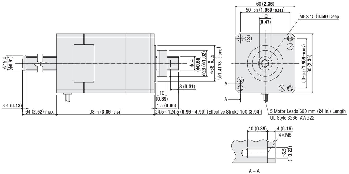
21 **DRL60PB4-05MG** (With electromagnetic brake)
