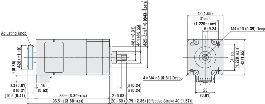
● The actuator comes with a motor lead wire/connector assembly [0.6 m (2 ft.)]. UL Style 3265, AWG24
