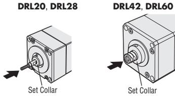
2. Holding the flat section of the screw shaft with a wrench, affix the load with a screw (or nut, in the case of the **DRL20** and **DRL28**).
