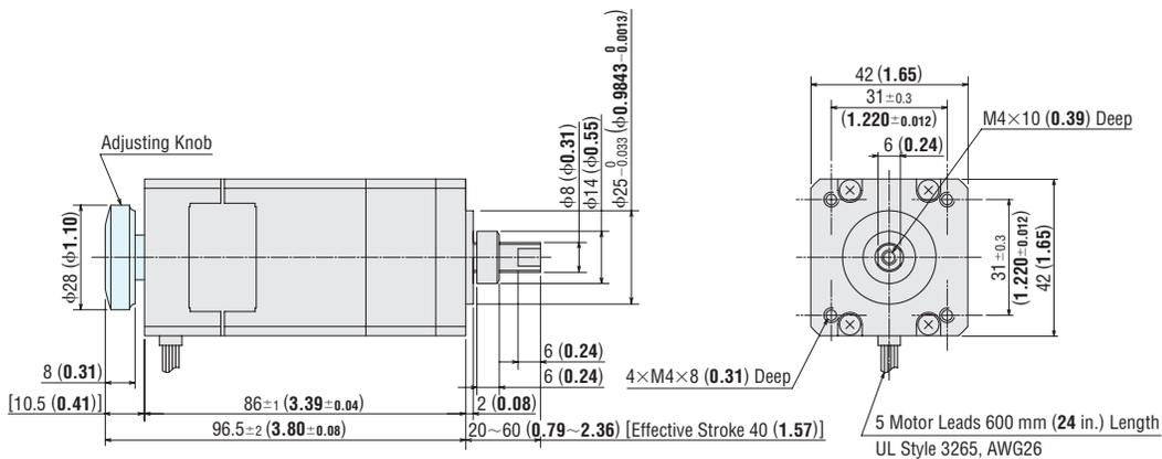
● Dimensions 14 and 16 apply to a configuration with adjusting knob. For models without adjusting knob, the shaft and adjusting knob shown in   areas should be ignored.
