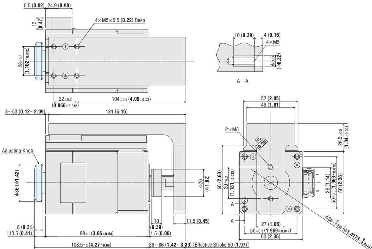
● The actuator comes with a motor lead wire/connector assembly [0.6 m (2 ft.)]. UL Style 3266, AWG22
