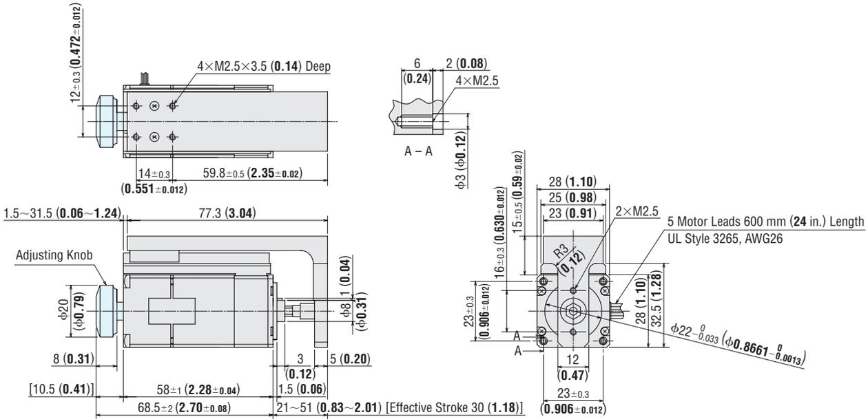
● Dimensions 22 and 23 apply to a configuration with adjusting knob. For models without adjusting knob, the shaft and adjusting knob shown in    areas should be ignored.
