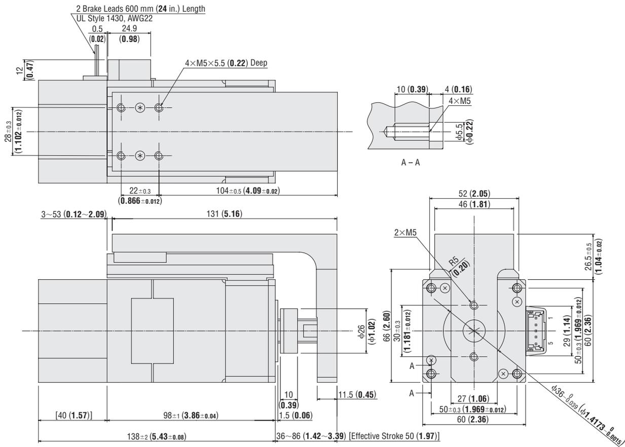
● The actuator comes with a motor lead wire/connector assembly [0.6 m (2 ft.)]. UL Style 3266, AWG22
