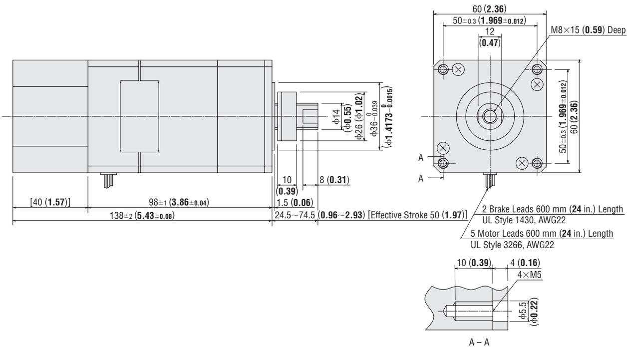
Ground Ball Screw/Rolled Ball Screw, Standard Motor, Guide Type
