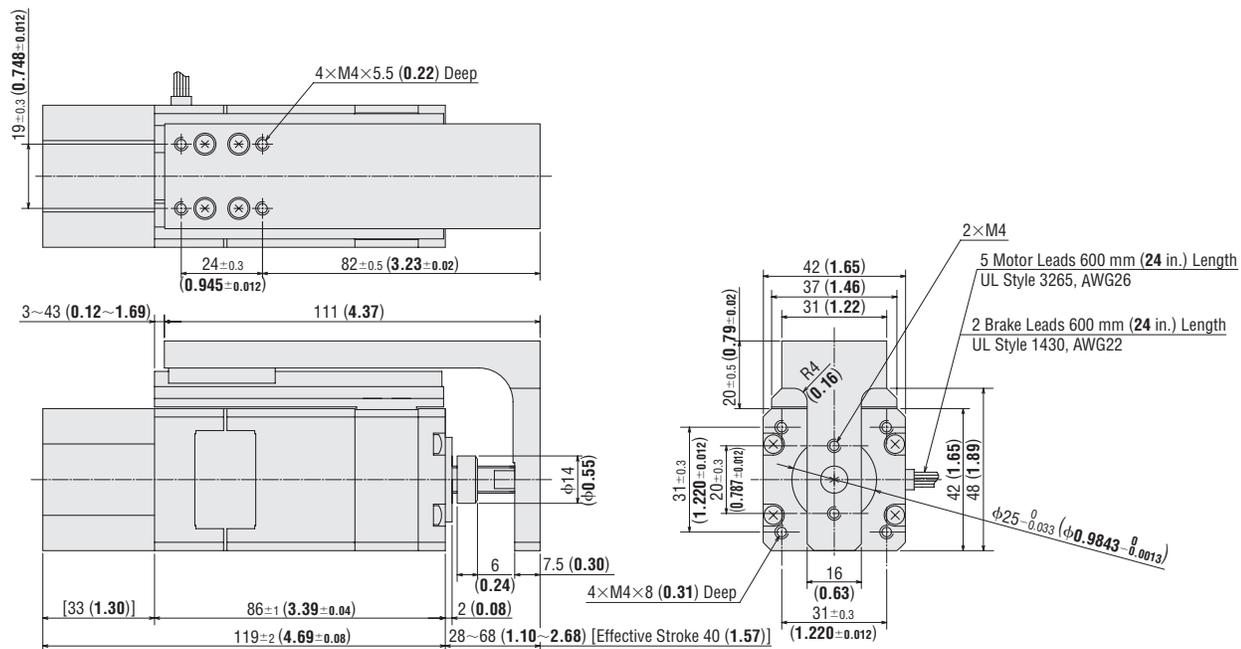
● Dimension 24 applies to a configuration with adjusting knob. For models without adjusting knob, the shaft and adjusting knob shown in  areas should be ignored.
