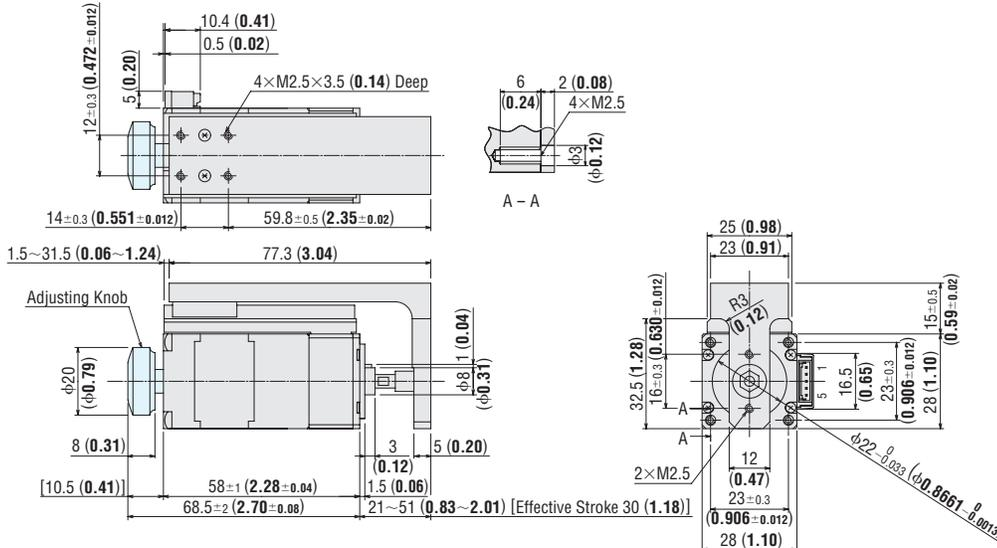
● The actuator comes with a motor lead wire/connector assembly [0.6 m (2 ft.)]. UL Style 3265, AWG24
