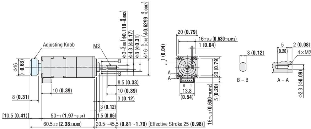
● The actuator comes with a motor lead wire/connector assembly [0.6 m (2 ft.)]. UL Style 3265, AWG24
