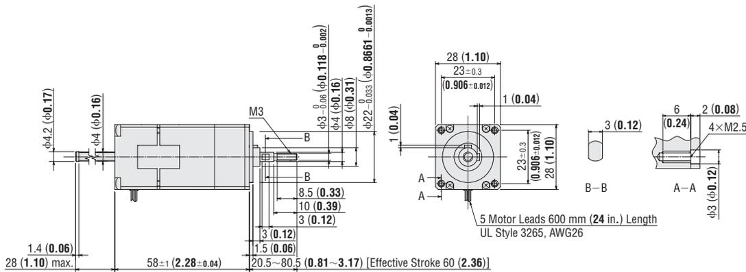
● Dimensions ① and ② apply to a configuration with adjusting knob. For models without adjusting knob, the shaft and adjusting knob shown in    areas should be ignored.
