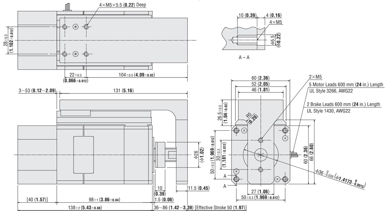
● Dimension 26 applies to a configuration with adjusting knob. For models without adjusting knob, the shaft and adjusting knob shown in blue areas should be ignored.
