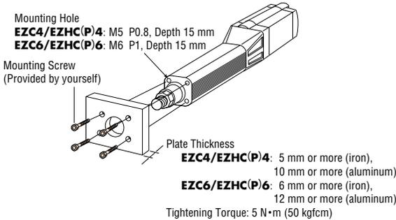
Installation using a cylinder flange **PAEZ□-F** (optional)
