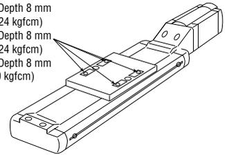
Note: The screws used to affix the load to the table shall not be longer than the thickness of the load by more than 8 mm. If the screw is more than 8 mm longer than the thickness of the load, the screw will contact the side cover of the slider.
