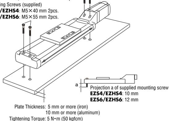
Mounting Hole: M5 P0.8, Depth 6 mm
