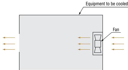
Fig. 1 Flow Path with Low Air Flow Resistance
