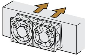
Fig. 5 Installing two fans
