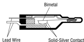
Fig. 13 Structure of Thermal Protector
