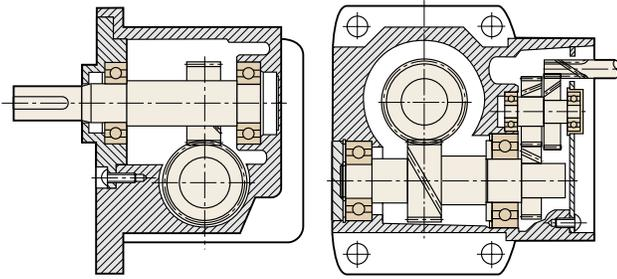
Structure of the Screw Gear
