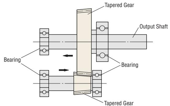
Structure of TH gear's final stage
