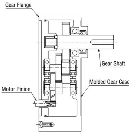
For use with general AC motors, many of which are fixed speed motors, the availability of various gear ratios suits a wide range of desired speeds. We support these motors with as many as 20 different gear ratios, ranging from 3:1 to 180:1.
