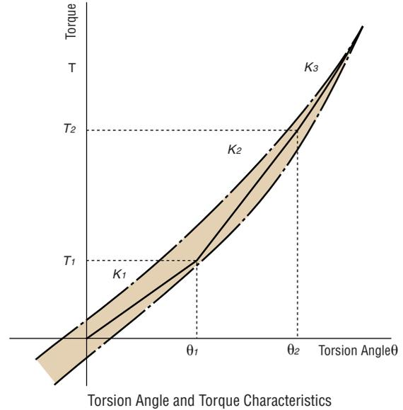
Torsion angles obtained by these equations are for individual harmonic gears.
