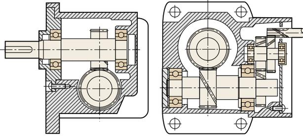
Structure of the Screw Gear
