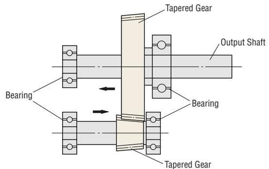
Structure of TH gear's final stage
