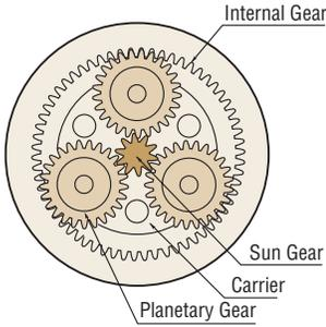
Cross Section of a **PN** Gear
