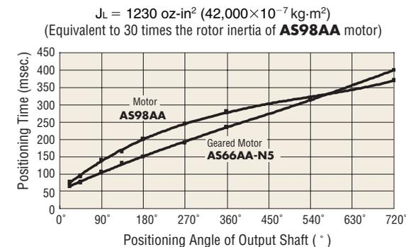
The geared motor is more effective in reducing the positioning time for a smaller positioning angle and a larger load inertia. The geared motor tends to achieve shorter positioning time in a wider range of positioning angles with a larger load inertia.
