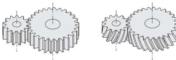
In both types of gearheads, the helical configuration is employed for the motor pinion and its mating gear. This contributes significantly to noise because of their high contact speeds, thereby achieving lower noise output.
