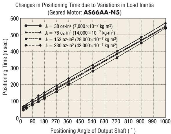
While the shortest positioning time of the motor changes significantly with the increase in load inertia, that of the geared motor shows little change. In other words, the geared motor is capable of driving a larger load inertia within the most consistent, shortest positioning time.
