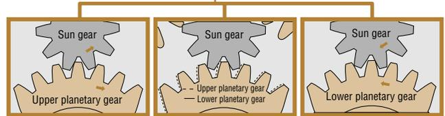
Relationship between upper and lower planetary gears
