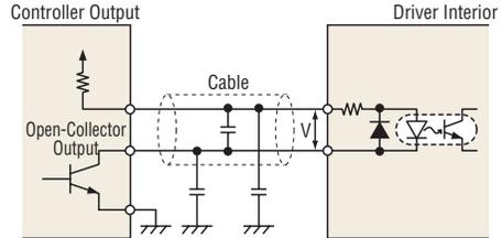
Image Diagram of Stray Capacitance in Cable
