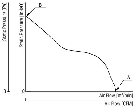
Fig. 14 Air Flow/Static Pressure Characteristics Curve
