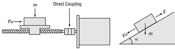
$$\tau_L = \left( \frac{FP_B}{2\pi\eta} + \frac{\mu_0 F_0 P_B}{2\pi} \right) \times \frac{1}{i} [\text{oz-in}] \dots\dots\dots ①$$
