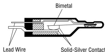
Fig. 13 Structure of Thermal Protector
