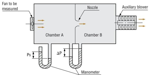
Fig. 4 Double-chamber Measuring Device
