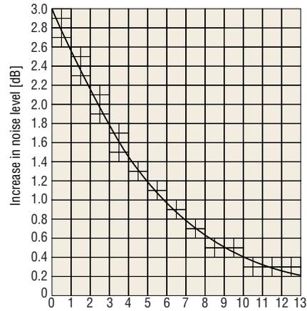
Fig. 10 Difference in Two Noise Levels
