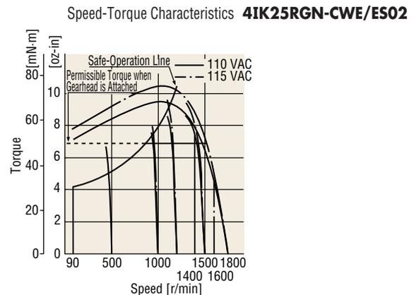
◆ **Safe Operation Line and Permissible Torque When Using a Gearhead**
