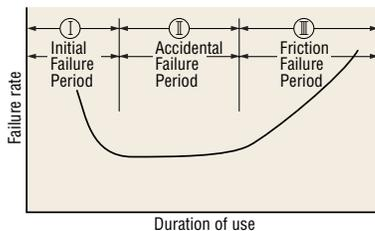
Fig. 11 Relationship between the Duration of Use and Failure Rate
