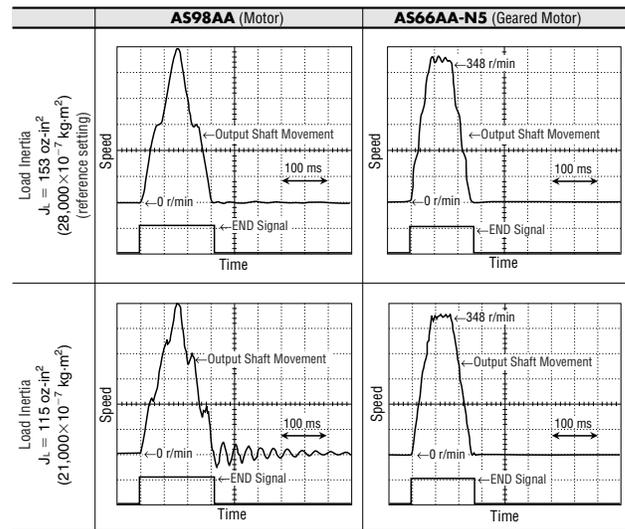
Even under the operating conditions that are optimized to reduce damping with a given load inertia, the damping characteristics of the motor will deteriorate with fluctuations in load inertia. For the motor it is therefore necessary to reset the operating conditions for optimal performance each time the load inertia fluctuates. On the other hand, the geared motor's damping characteristics change little with fluctuations in load inertia, thereby ensuring steady operation.
