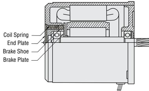
The brake mechanism is constructed as shown in the figure above. The coil spring applies constant pressure to allow the brake shoe to slide toward the brake plate. This mechanism provides a certain degree of holding brake force, but the force is limited due to the mechanism's structure, as described above. The brake force produced by the brake mechanism of an Oriental Motor reversible motor is approximately 10% of the motor's output torque.
