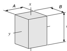
$$J_x = \frac{1}{12} m (A^2 + B^2) = \frac{1}{12} \rho A B C (A^2 + B^2) [\text{oz-in}^2] \dots\dots\dots ⑫$$
