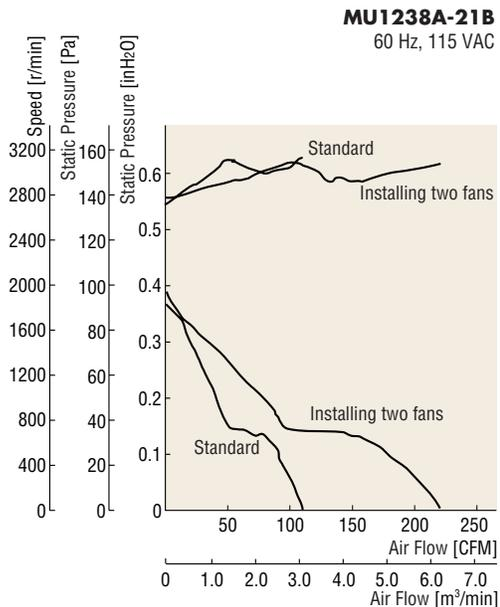
Fig. 6 Changes in fan characteristics of static pressure and amount of air flow
