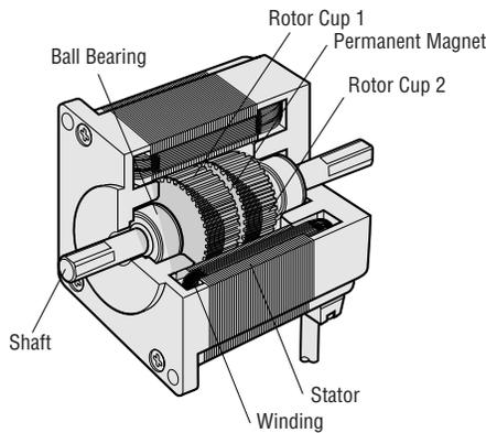
Motor Structural Diagram 1: Cross-Section Parallel to Shaft
