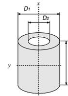
$$J_x = \frac{1}{8} m (D_1^2 + D_2^2) = \frac{\pi}{32} \rho L (D_1^4 - D_2^4) [\text{oz-in}^2] \dots\dots\dots ⑨$$
