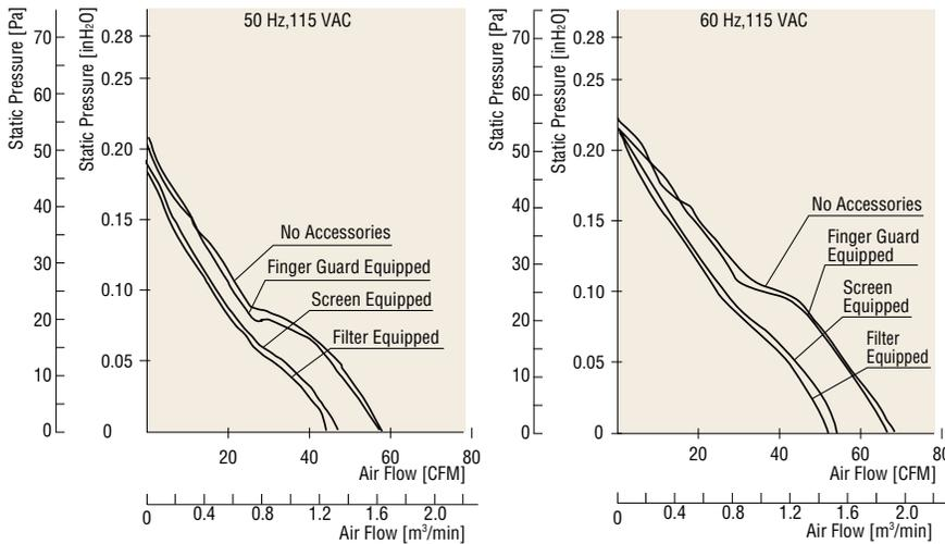
Fig. 8 Changes in Characteristics with Optional Parts Attached to the **MU1225S-21**
