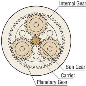
Cross Section of a PN Gear
