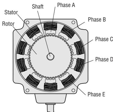
Motor Structural Diagram 2: Cross-Section Perpendicular to Shaft
