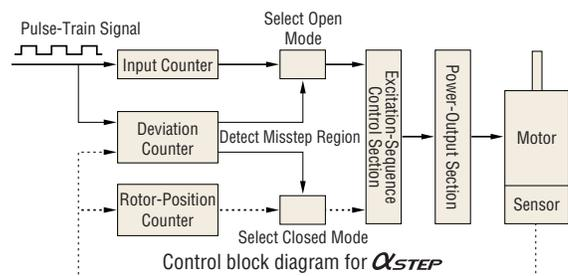
Rotor position counter: Specifies an excitation sequence that would develop maximum torque for a given rotor position.
