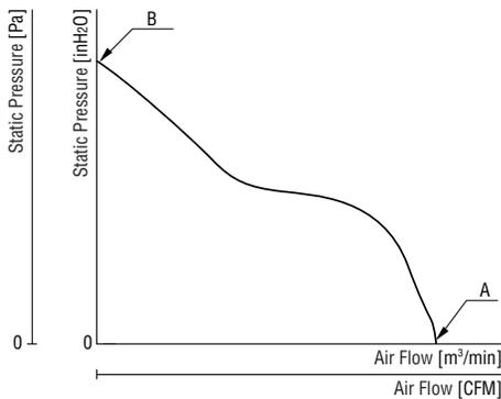
Fig. 14 Air Flow/Static Pressure Characteristics Curve
