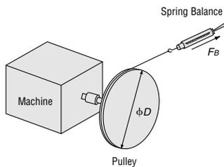
$$\tau_L = \frac{F_B D}{2} [\text{oz-in}] \dots\dots\dots ⑥$$
