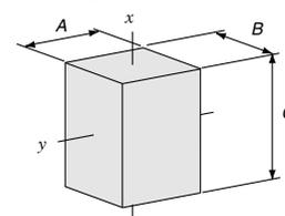
$$J_x = \frac{1}{12} m (A^2 + B^2) = \frac{1}{12} \rho A B C (A^2 + B^2) [\text{oz-in}^2] \dots\dots\dots ⑫$$
