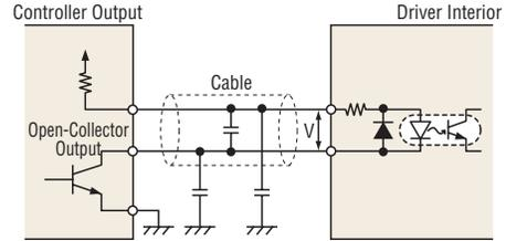
Image Diagram of Stray Capacitance in Cable
