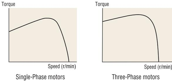
Induction motors are available in two types: single-phase (capacitor run) and three-phase induction motors. With the single-phase motor, the starting torque is generally smaller than the operating torque, while the three-phase motor features a relatively greater starting torque.
