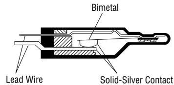
Fig. 13 Structure of Thermal Protector
