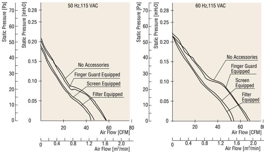
Fig. 8 Changes in Characteristics with Optional Parts Attached to the MU12255-21
