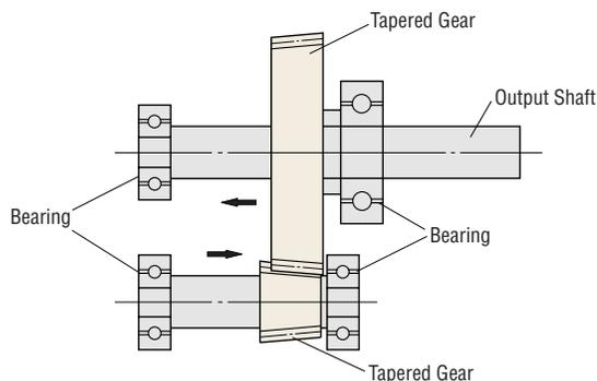
Structure of TH gear's final stage
