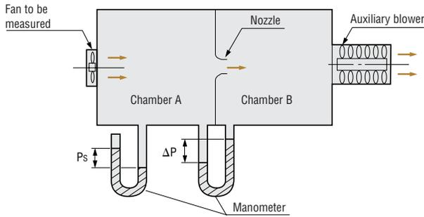
Fig. 4 Double-chamber Measuring Device
