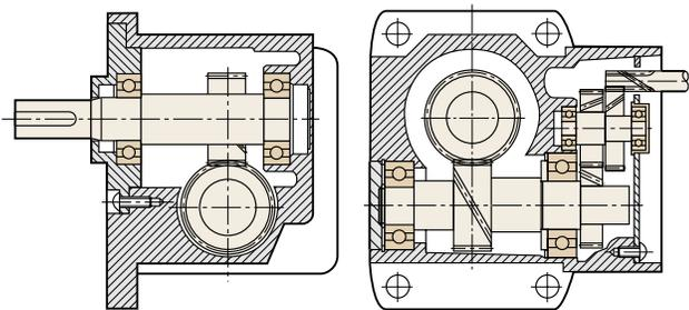
Structure of the Screw Gear
