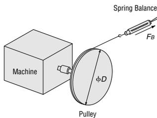
$$\tau_L = \frac{F_B D}{2} [\text{oz-in}] \dots\dots\dots ⑥$$
