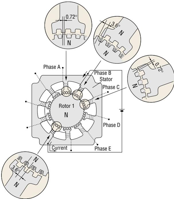
In other words, when excitation switches from phase A to B, the rotor rotates by 0.72°. As excitation shifts from phase A, to phases B, C, D and E, then back around to phase A, the stepping motor rotates precisely in 0.72° steps.
