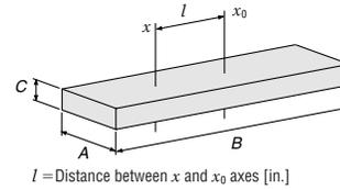
$$J_x = J_{x_0} + m l^2 = \frac{1}{12} m (A^2 + B^2 + 12 l^2) [\text{oz-in}^2] \dots\dots\dots ⑪$$
