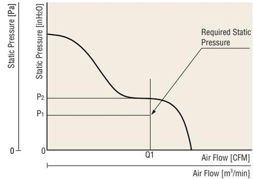
Fig. 3 Air Flow vs. Static Pressure Characteristics Curve
