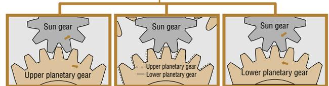
Relationship between upper and lower planetary gears
