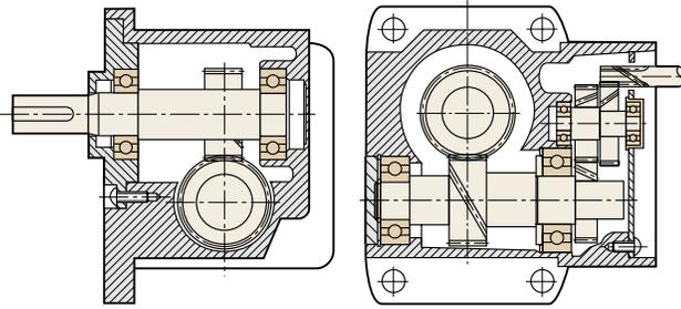
Structure of the Screw Gear
