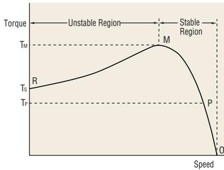
Under conditions of no load, the motor rotates at a speed close to synchronous rotation (O). As the load increases, the motor's speed drops to a level (P) where a balance is achieved between load and motor torque ( $T_p$ ).
