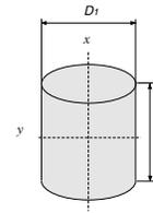
$$J_x = \frac{1}{8} m D_1^2 = \frac{\pi}{32} \rho L D_1^4 [\text{oz-in}^2] \dots\dots\dots ⑦$$
