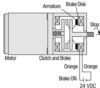
The figure below shows the relationship between the action of the motor shaft and output shaft and the state of excitation of the clutch and brake coils.
