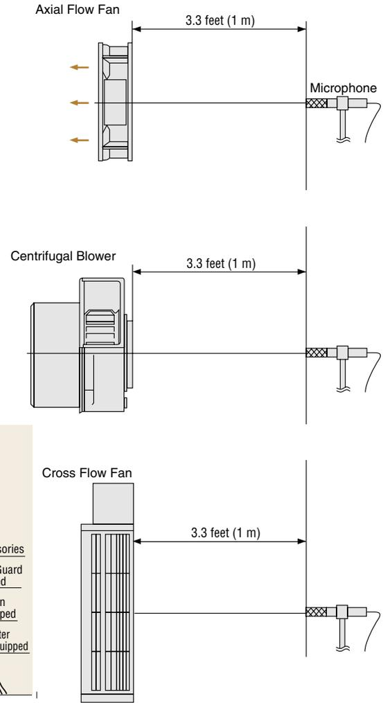
Fig. 9 Measurement of Fan Noise
