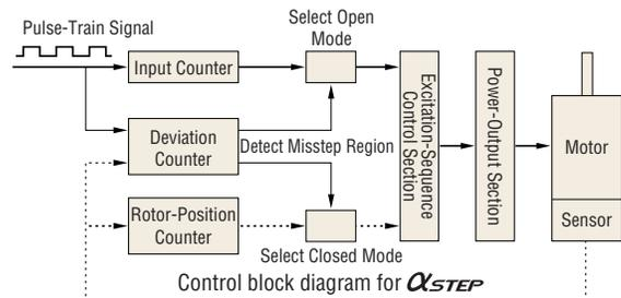
Rotor position counter: Specifies an excitation sequence that would develop maximum torque for a given rotor position.
