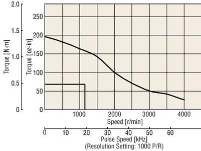
Select a motor for which the required torque falls within the pull-out torque of the speed-torque characteristics.
