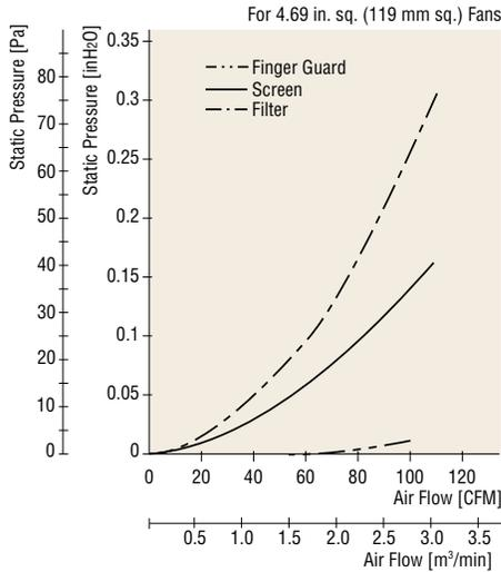
Fig. 7 Changes in Characteristics with Optional Parts
