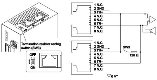
\* The GND line is used in common with CN1 (not insulated).
