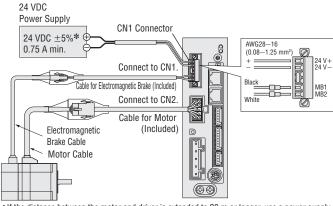
stIf the distance between the motor and driver is extended to 20 m or longer, use a power supply of 24 VDC  $\pm$ 4%.
