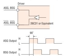
A counter or similar device can be connected to monitor the position of the motor. The pulse resolution is the same as the motor resolution at the time of power-on.
