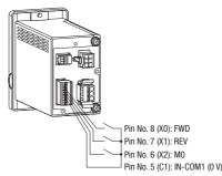
Applicable Lead Wire Size AWG26~20 (0.14~0.5 mm<sup>2</sup>)
