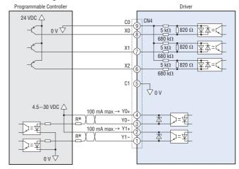
\*Recommended Resistance Value 24 VDC: 680  $\Omega$ ~2.7 k $\Omega$  (2 W)
