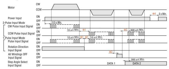
The shaded section indicates that the photocoupler is on.  $\square$
