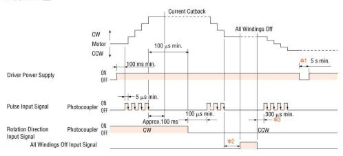
Note: 100 µs or more is the standard interval time for switching from CW to CCW. Note that the interval time varies greatly depending on the motor and load inertia.
