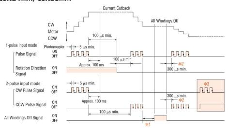
Note: 100 µs or more is the standard interval time for switching from CW to CCW. Note that the interval time varies greatly depending on the motor and load inertia.
